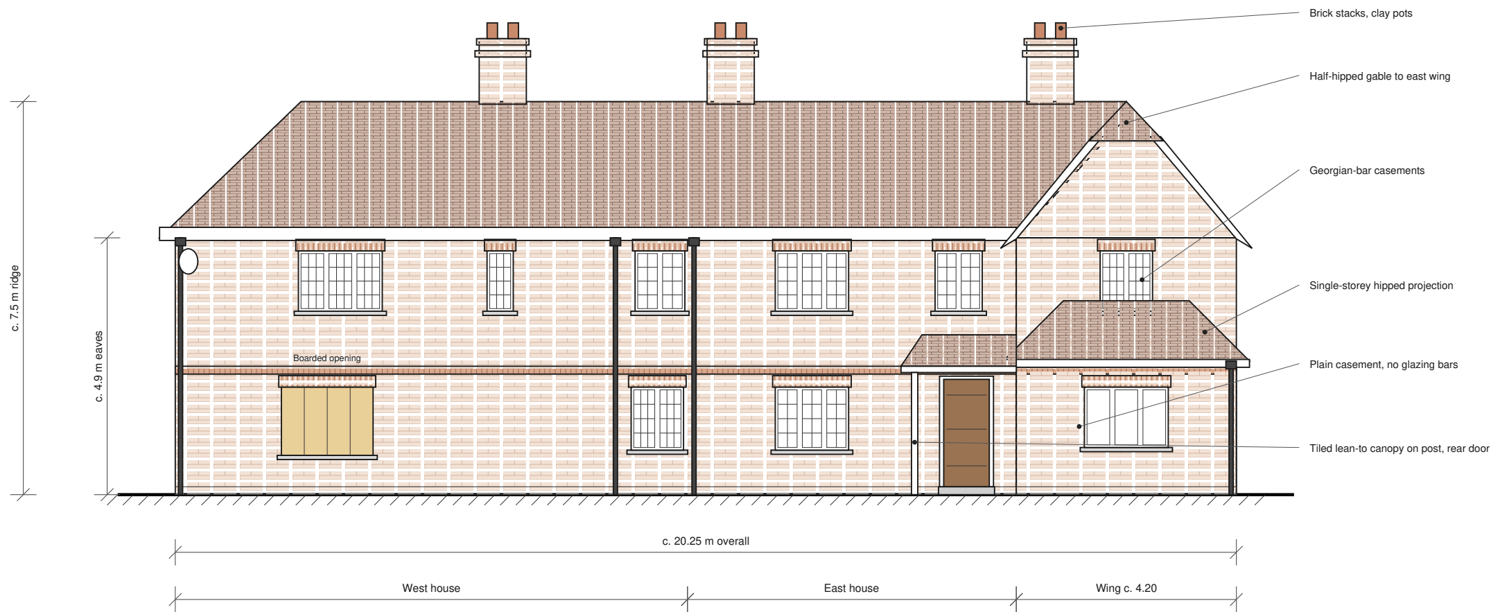
NORTH (FRONT) ELEVATION
