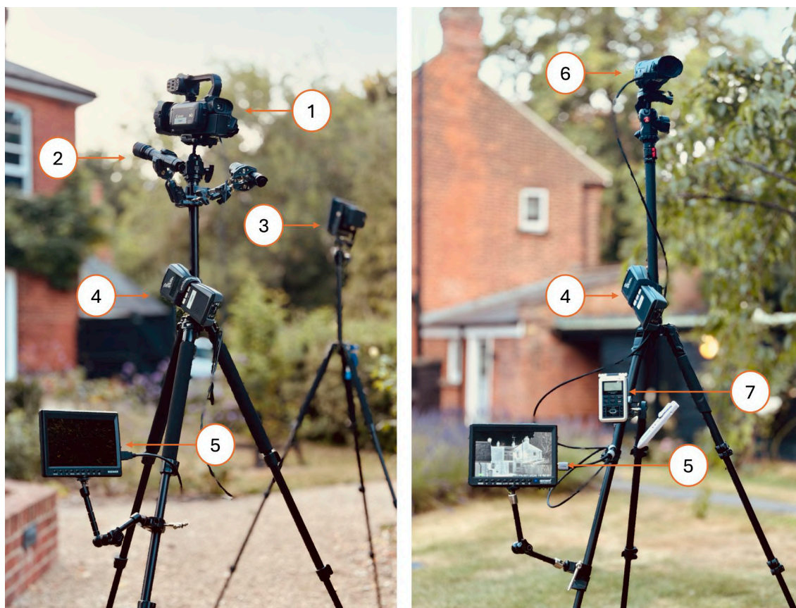
Photo 1. Infrared (left) and thermal imaging (right) Night Vision Aids (NVAs).
