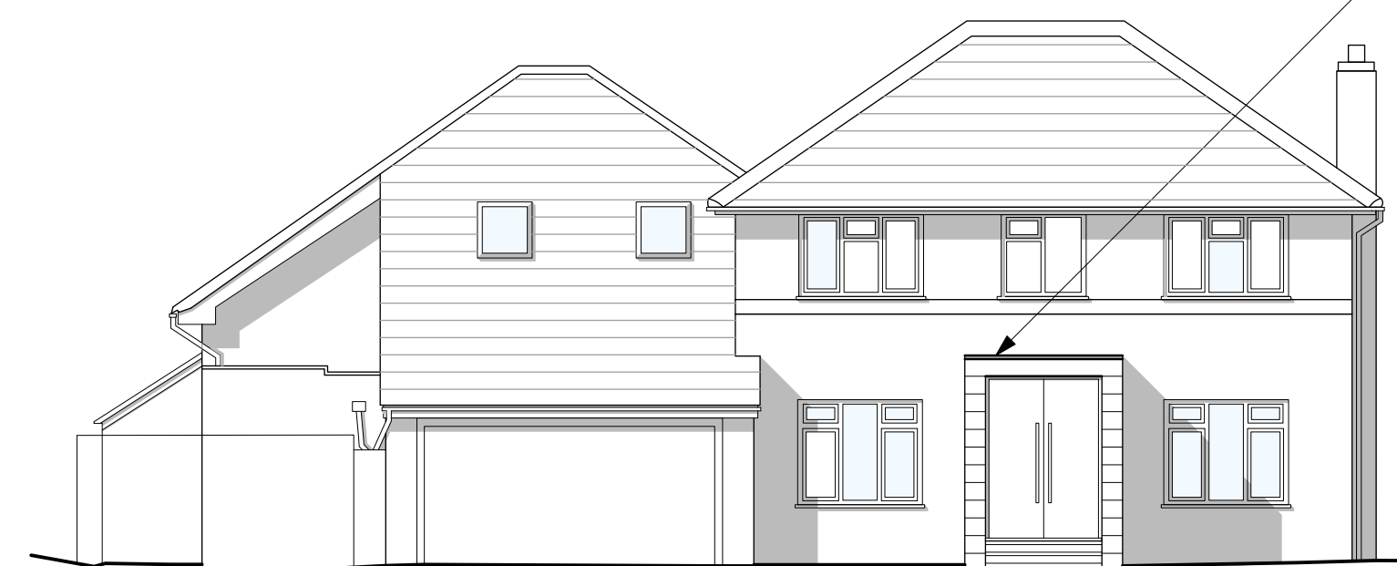
Front Elevation - showing new porch.
