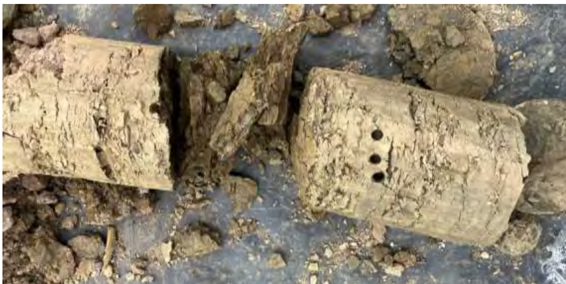
Figure 5-H: Photograph of the typical Wadhurst Clay Formation encountered in WS05
