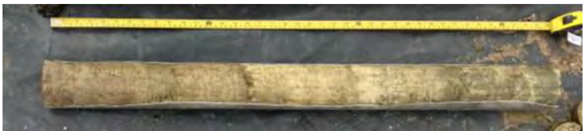
Figure 5-G: Photograph of the Wadhurst Clay Formation encountered in WS04
