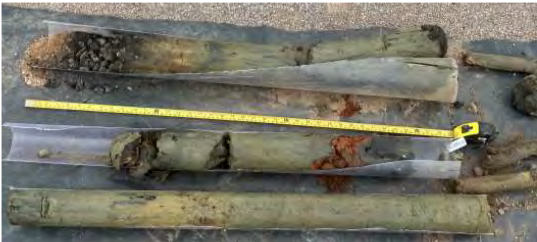
Figure 5-C: Made Ground encountered in WS03
