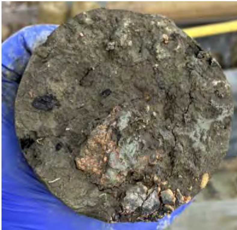
Figure 5-D: Made Ground excavated from WS01
