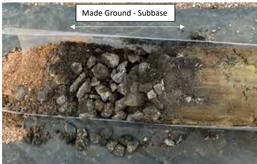
Figure 5-B: Made Ground – Subbase encountered in WS03
