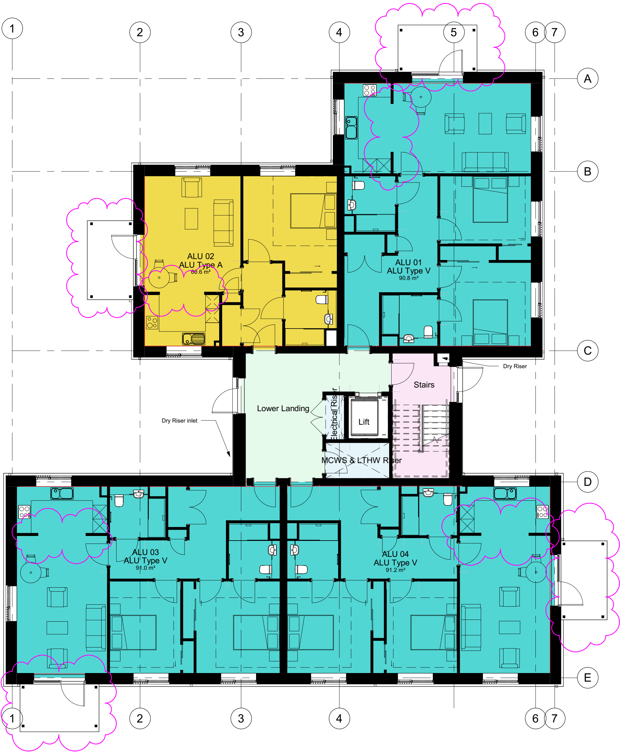
Proposed Ground Floor Plan 1 : 100
