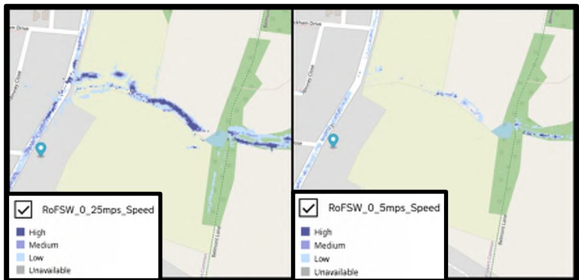
Figure 9 – Risk of surface water flooding velocity of approx. 0.25 m/s (left) and approx. 0.5 m/s (right).
