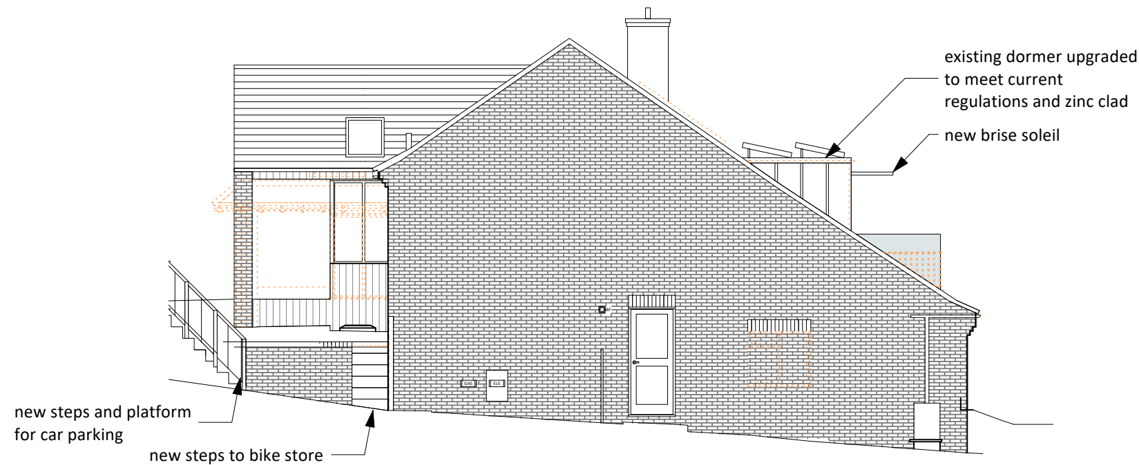
2 Proposed Side Elevation (NW) Scale: 1:100
