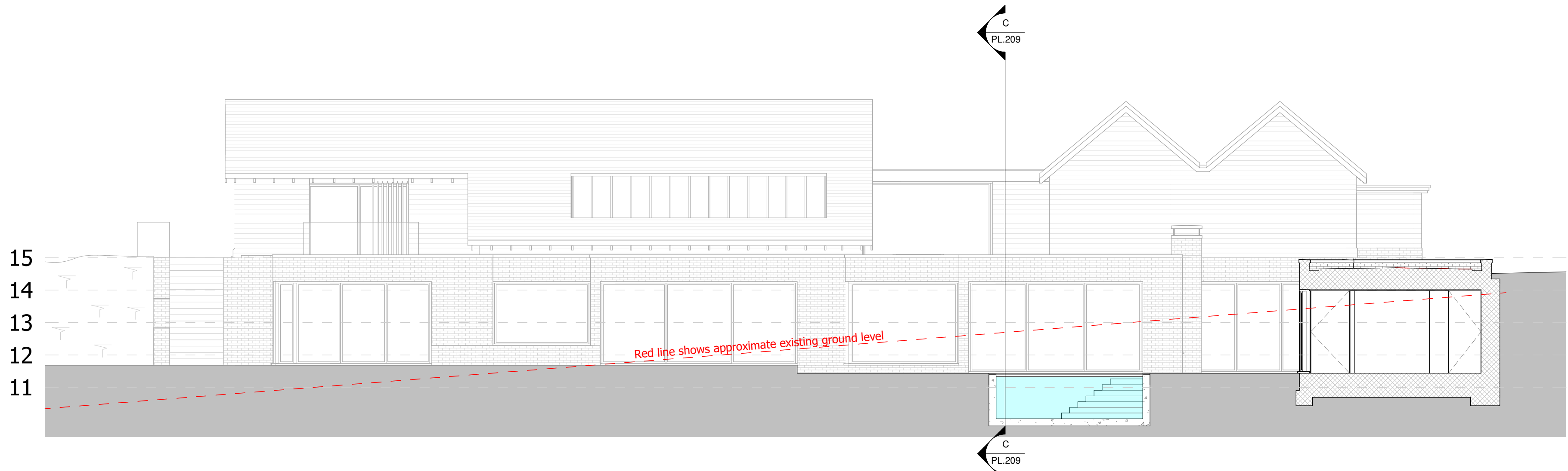
Site Section B-B - North - South 1 : 100
