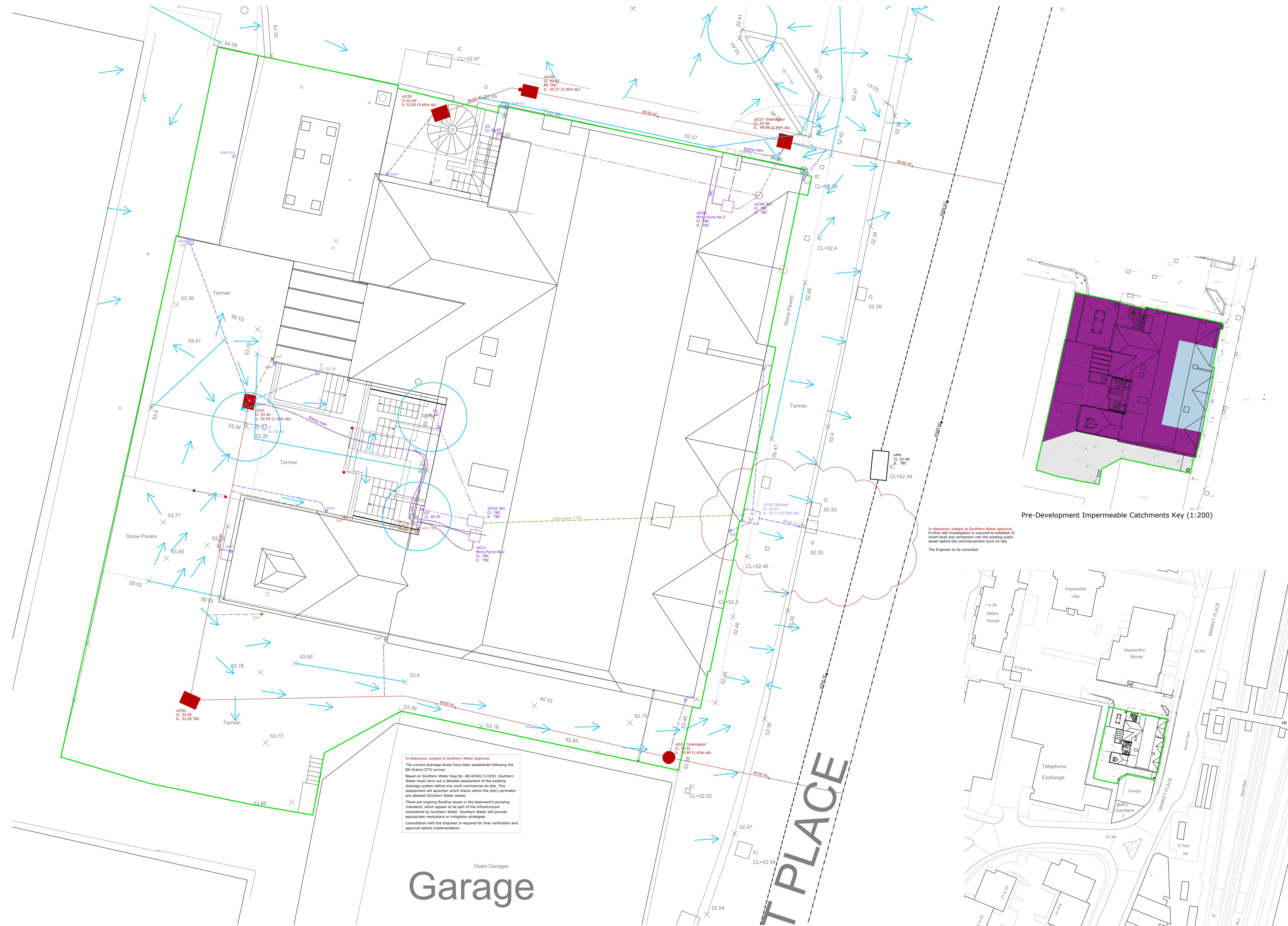
Site Plan Showing Existing Drainage Survey (1:500)
