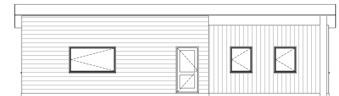
Existing South Elevation 1:100 @ A1
