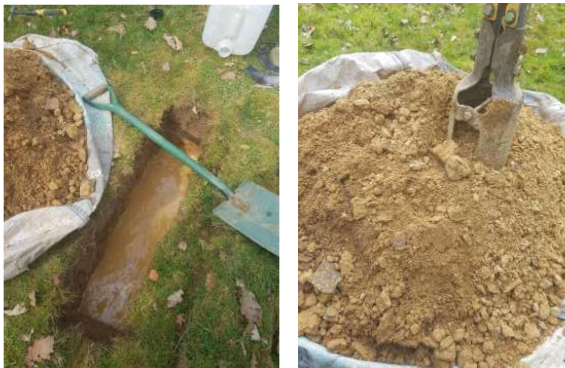
Fig 3. Soakaway test photos
