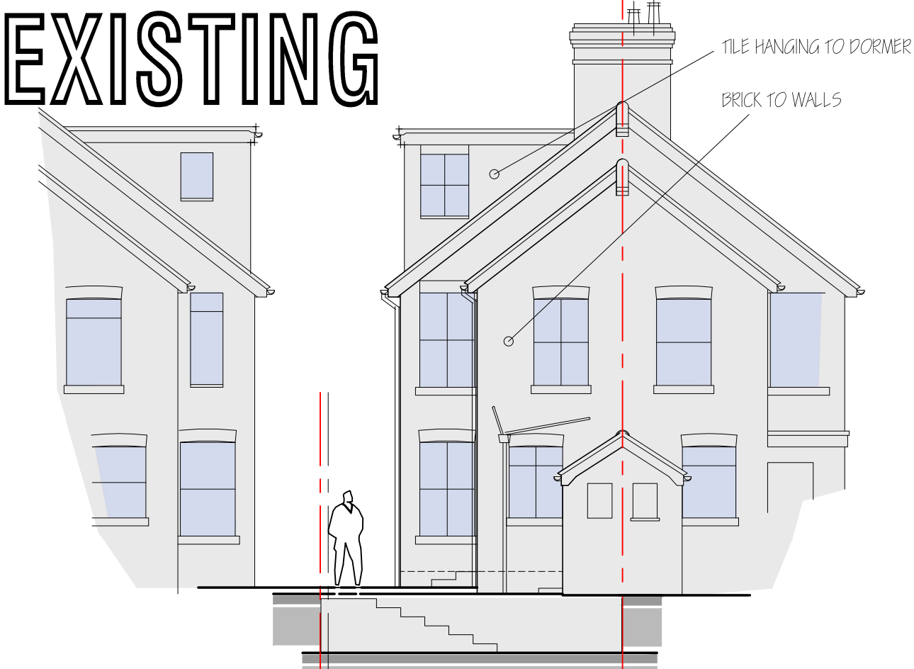
Existing Rear (South) Elevation
