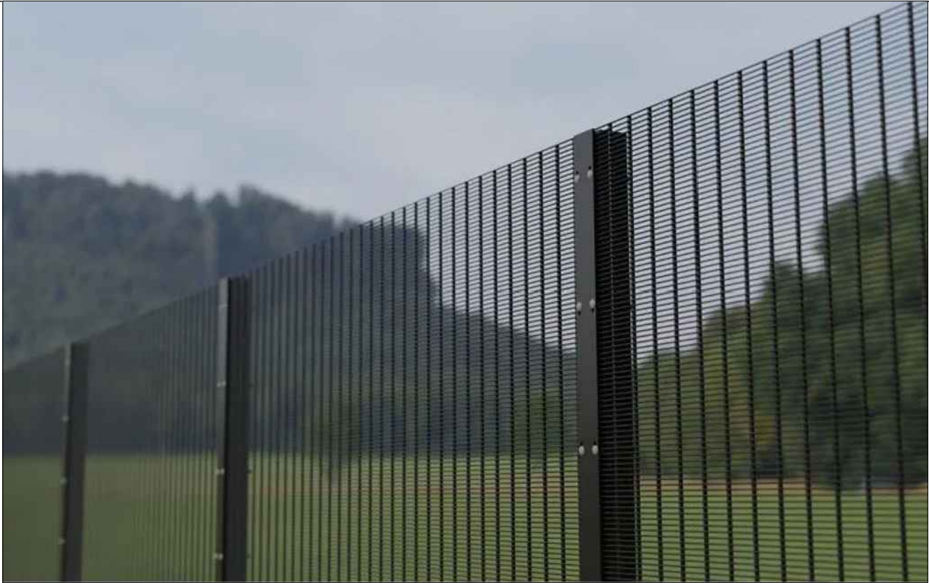
Image from CLD Systems website Image illustrates product with an LPS 1175 security rating of B3 (SR2). Note single layer of mesh (permitted by use of heavier 10mm vertical bars) and the bolted strap plates on each post. This system may be deployed using off-site assembled modules
