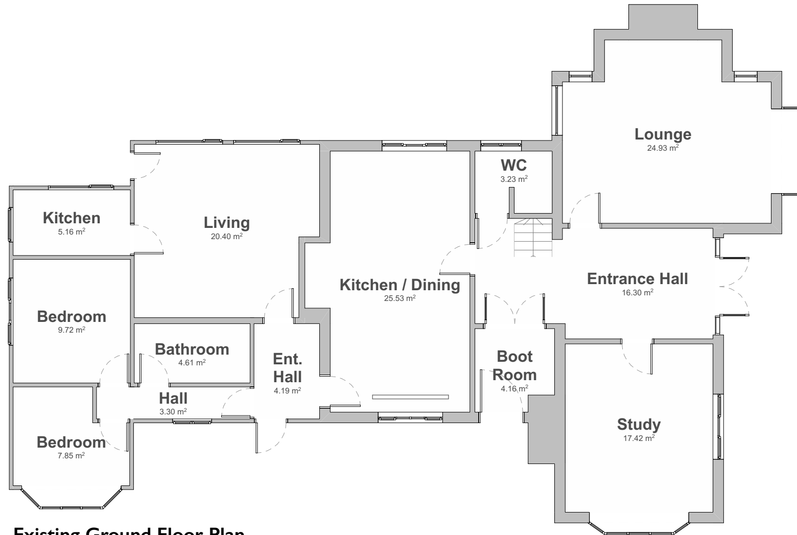
Existing Ground Floor Plan Scale 1:100 @ A3
