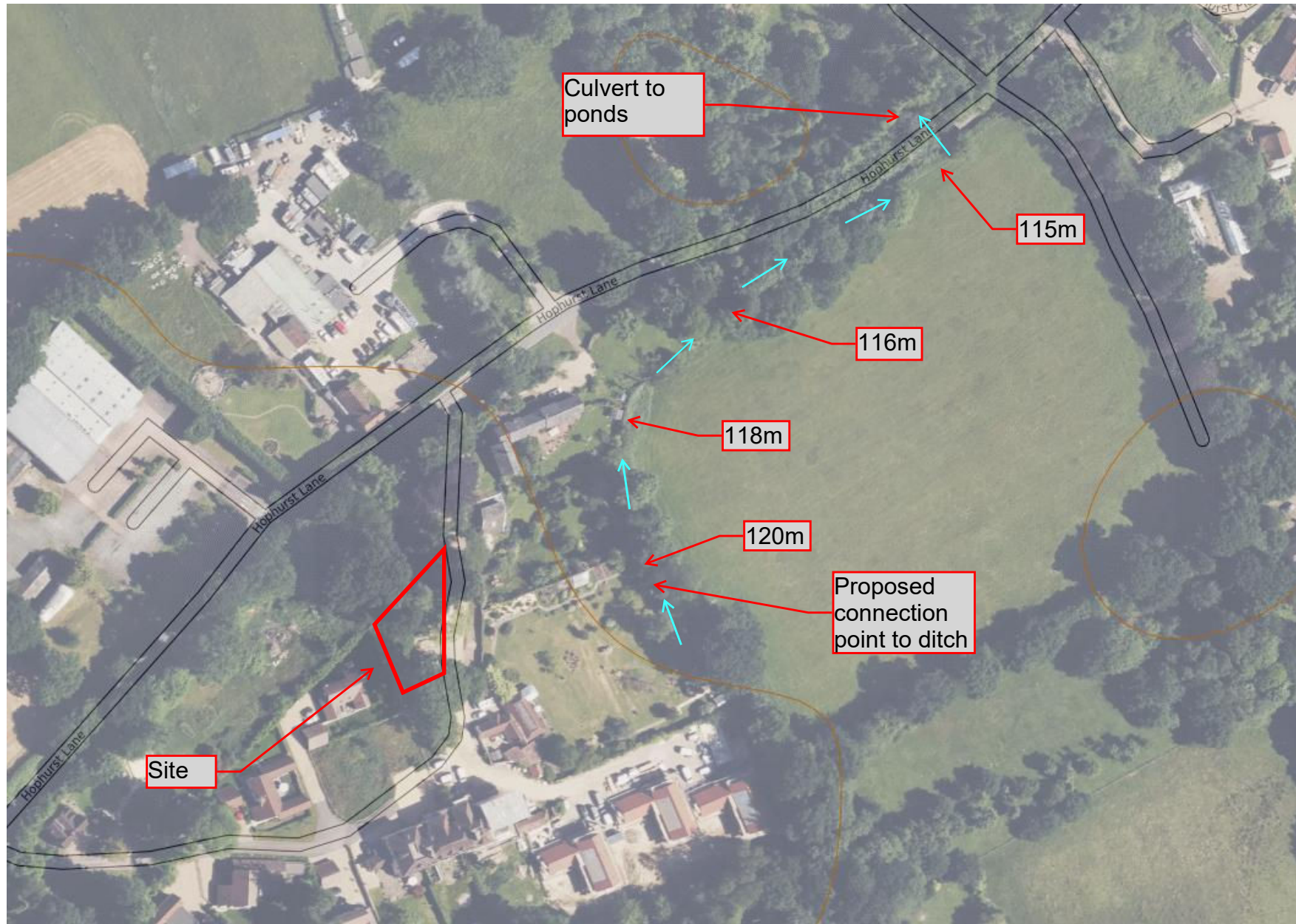
Existing Ditch Levels
