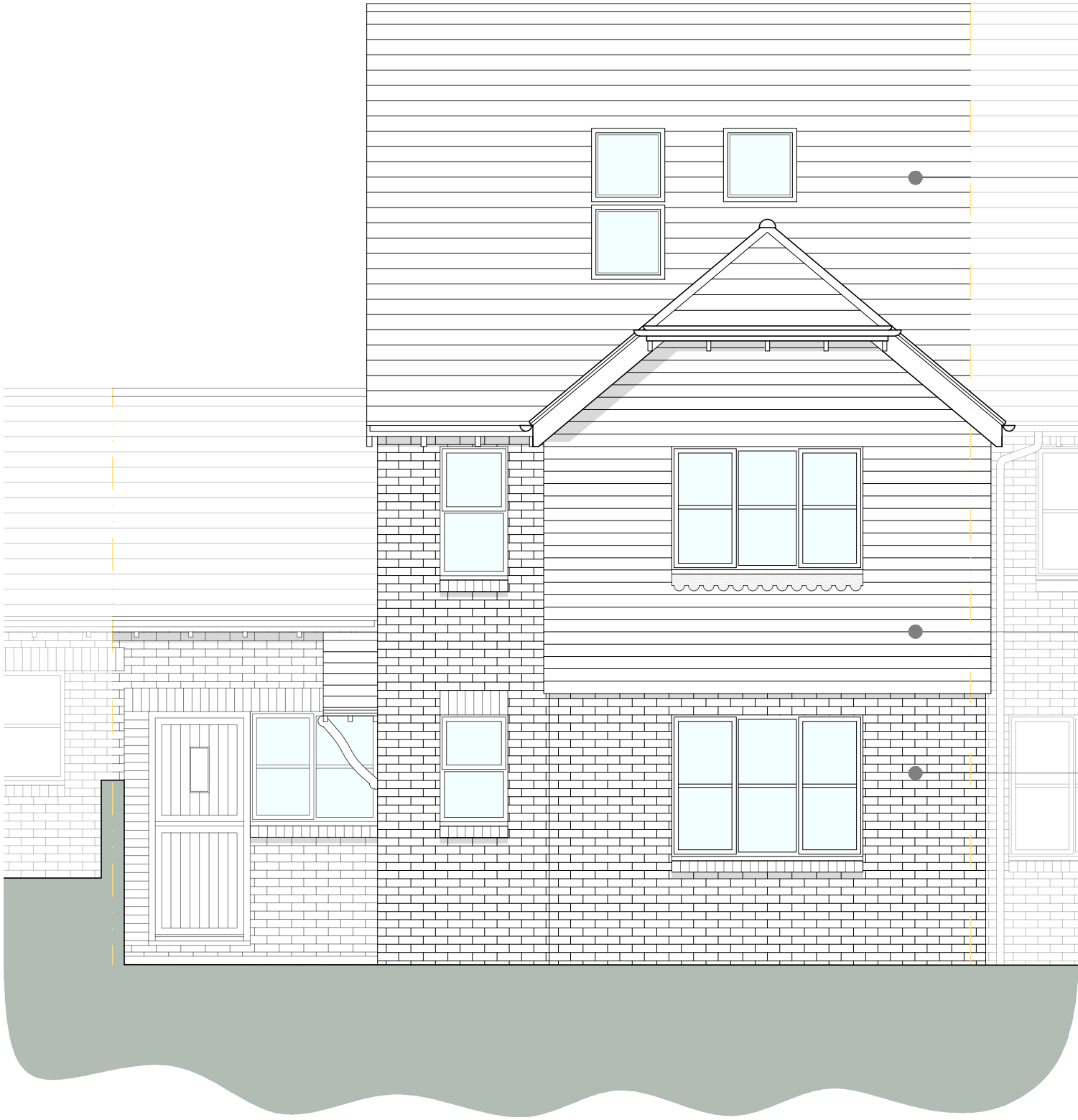
existing north-west elevation 1:50
