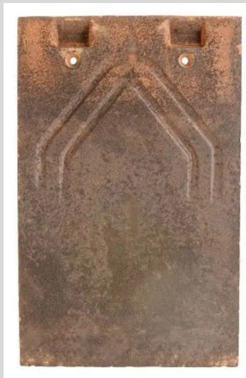
Image 14 - Edilians Phalempin Weathered machine made tile
