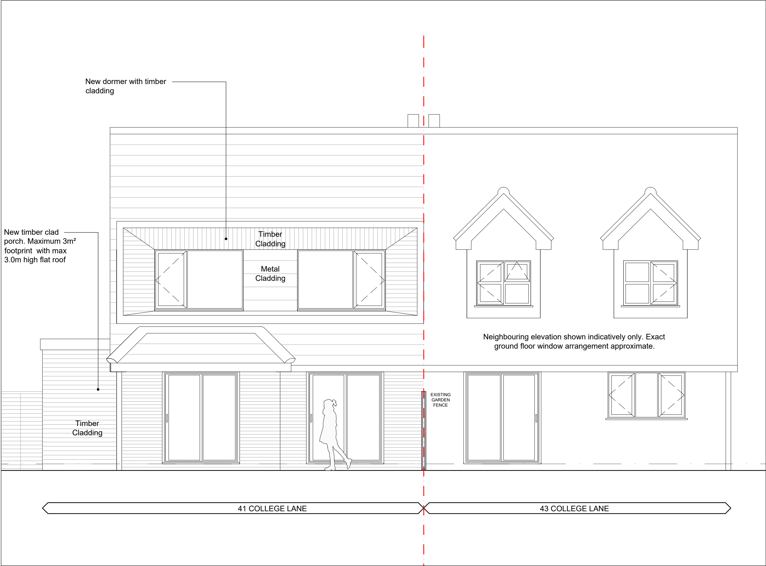
02 North Elevation (Rear) Scale 1:50@A1 / 1:100@A3
