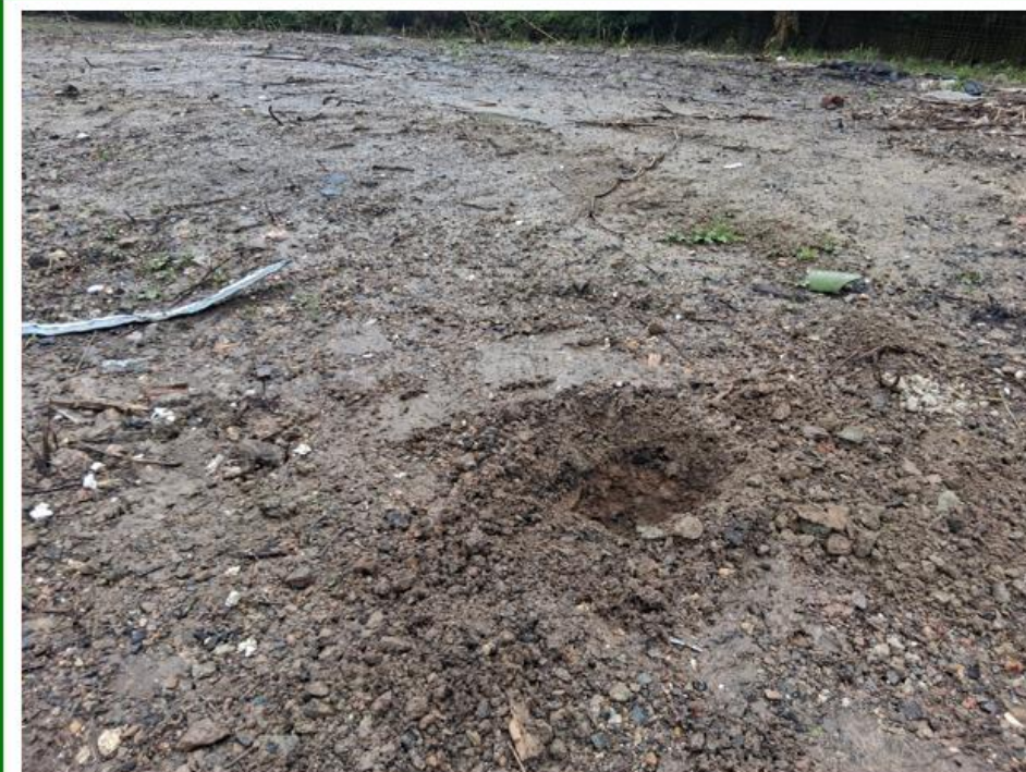
Photo No.8: IP04 showing made ground deposits associated with the former nursery usage adj. to site
