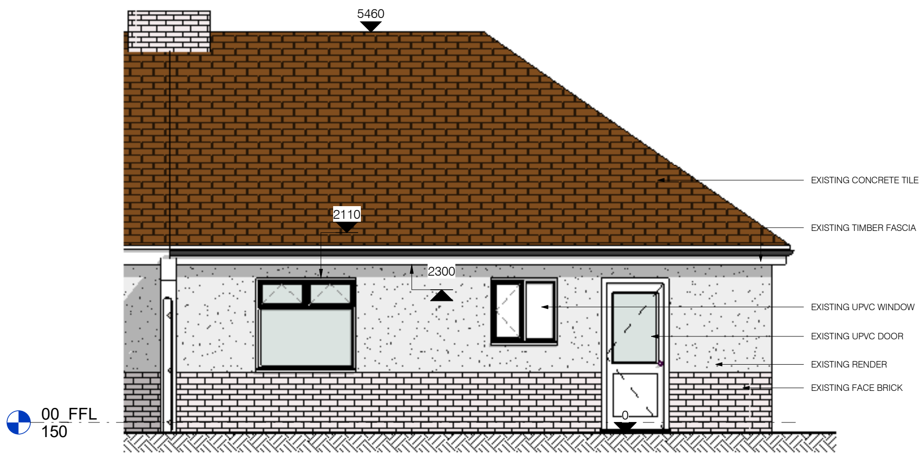
3 EXISTING SOUTH ELEVATION 1 : 50
