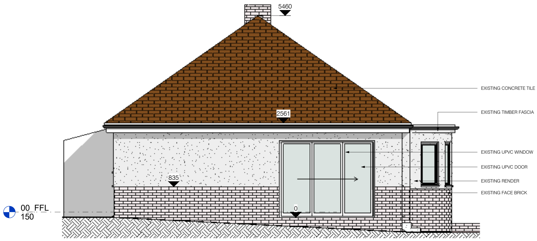
2 EXISTING EAST ELEVATION 1 : 50
