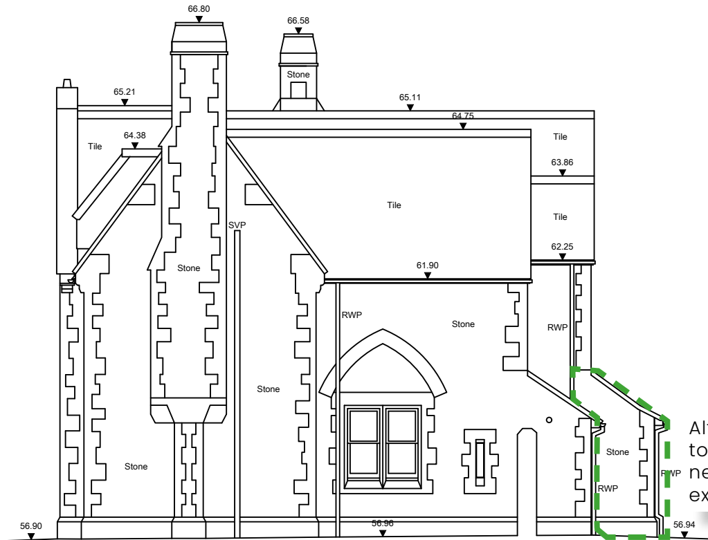
Existing East Elevation
