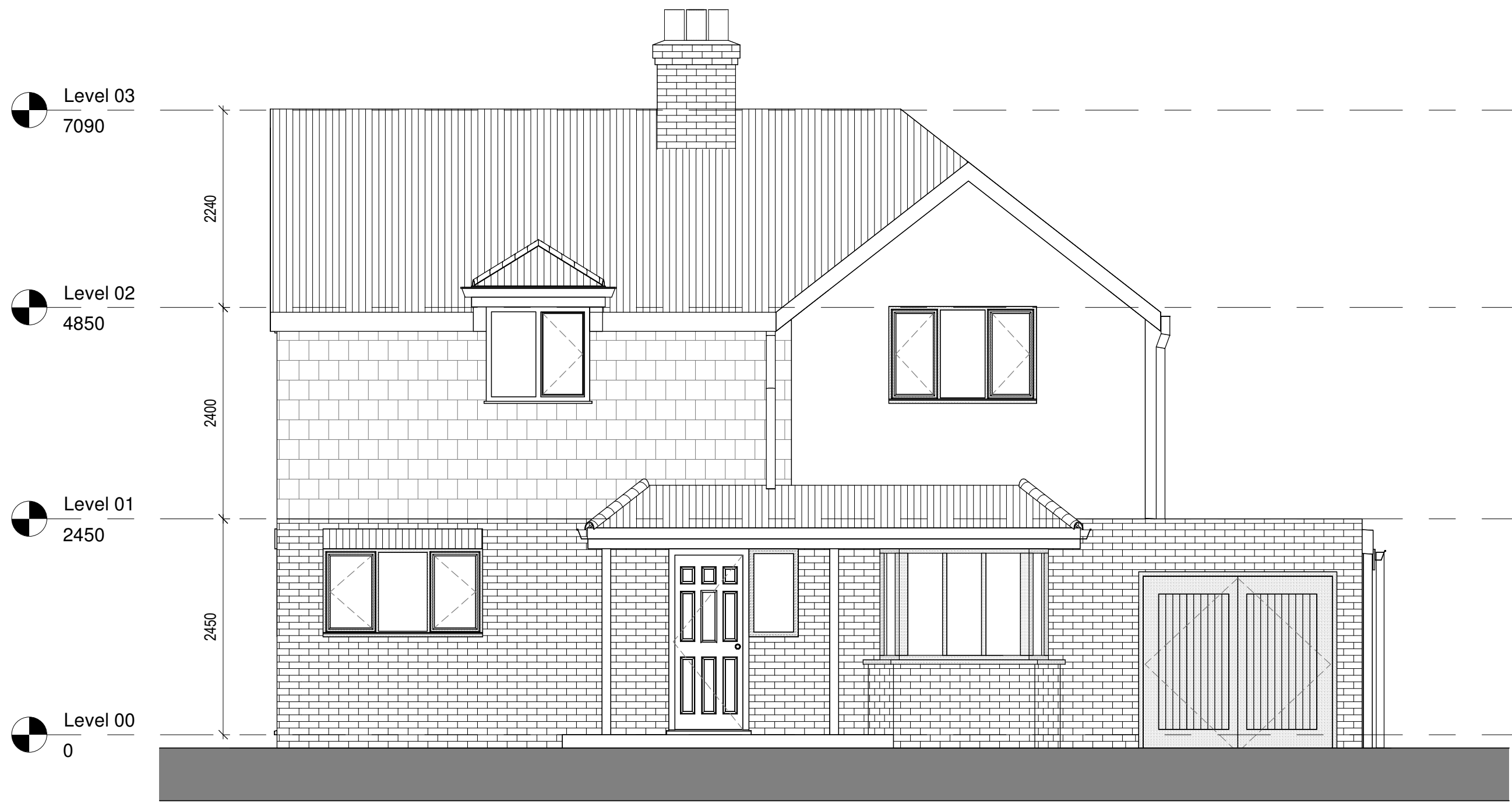
1 Front Elevation - Existing 1 : 50
