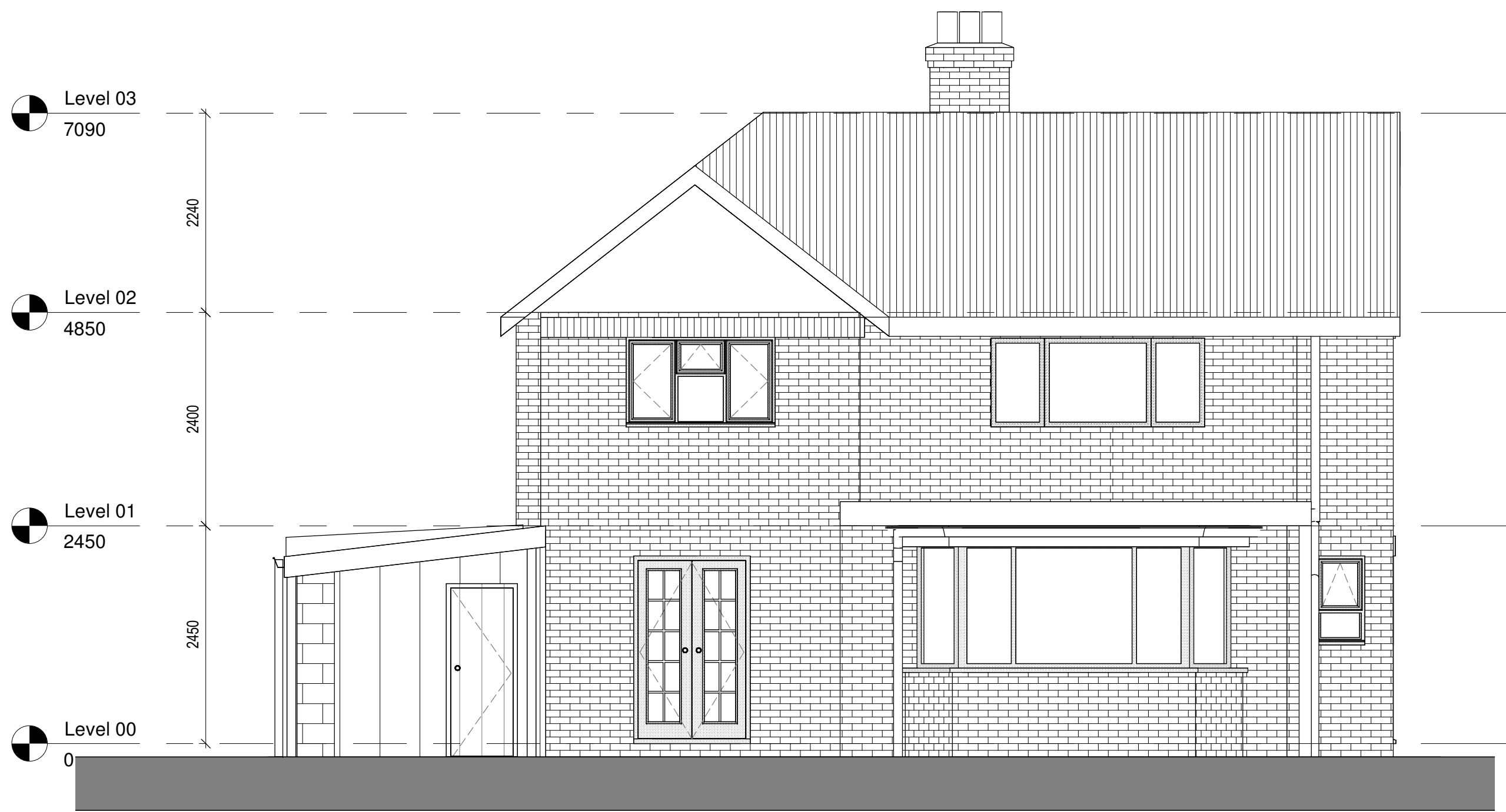
3 Rear Elevation - Existing 1 : 50
