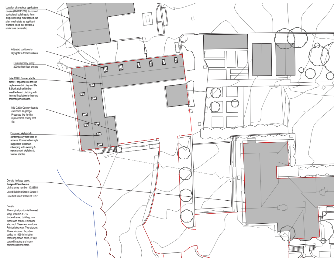
Proposed block plan (not to scale)
