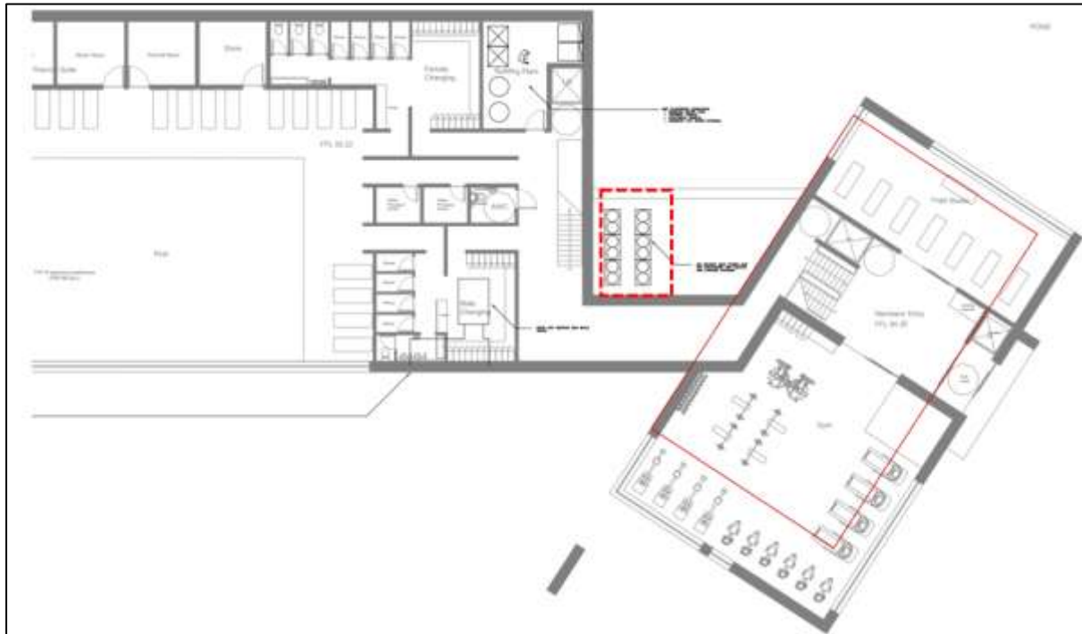
Figure 13. Location of Air Source Heat Pumps
