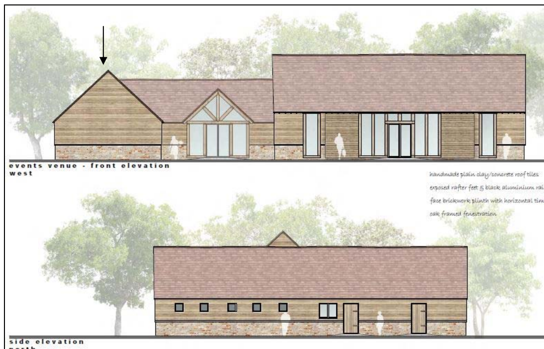
Plate 21: Extract of the proposal scheme drawings prepared by G3 Architecture showing the blank western end and low storey height of the north ancillary range (arrow)
