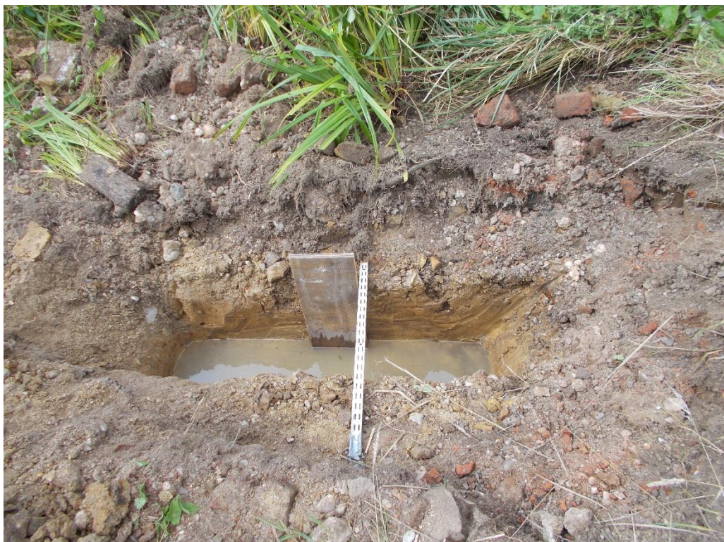
Photo 6: Percolation Test Pit PTP 2.
