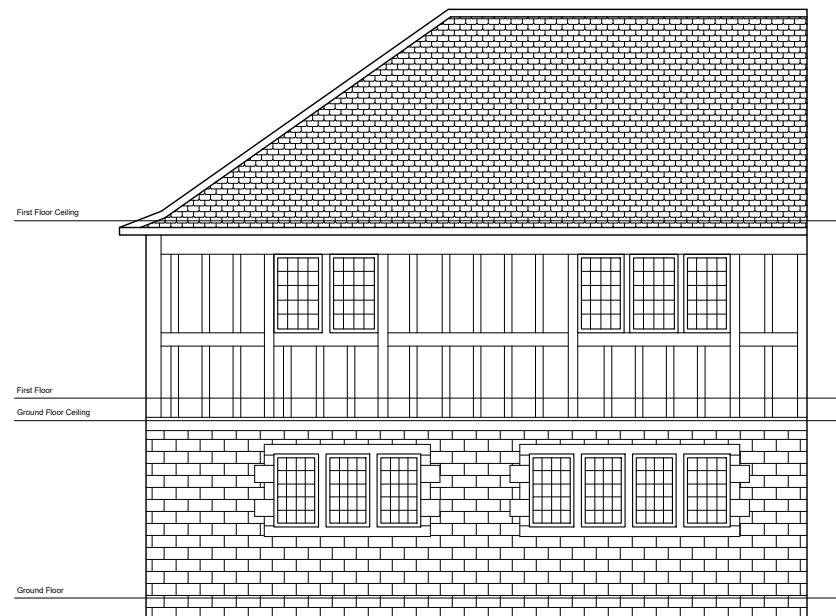
FRONT ELEVATION AS EXISTING
