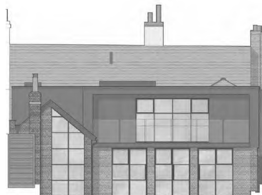
Proposed enhanced visibility of the historic outrigger - original brickwork walls exposed
