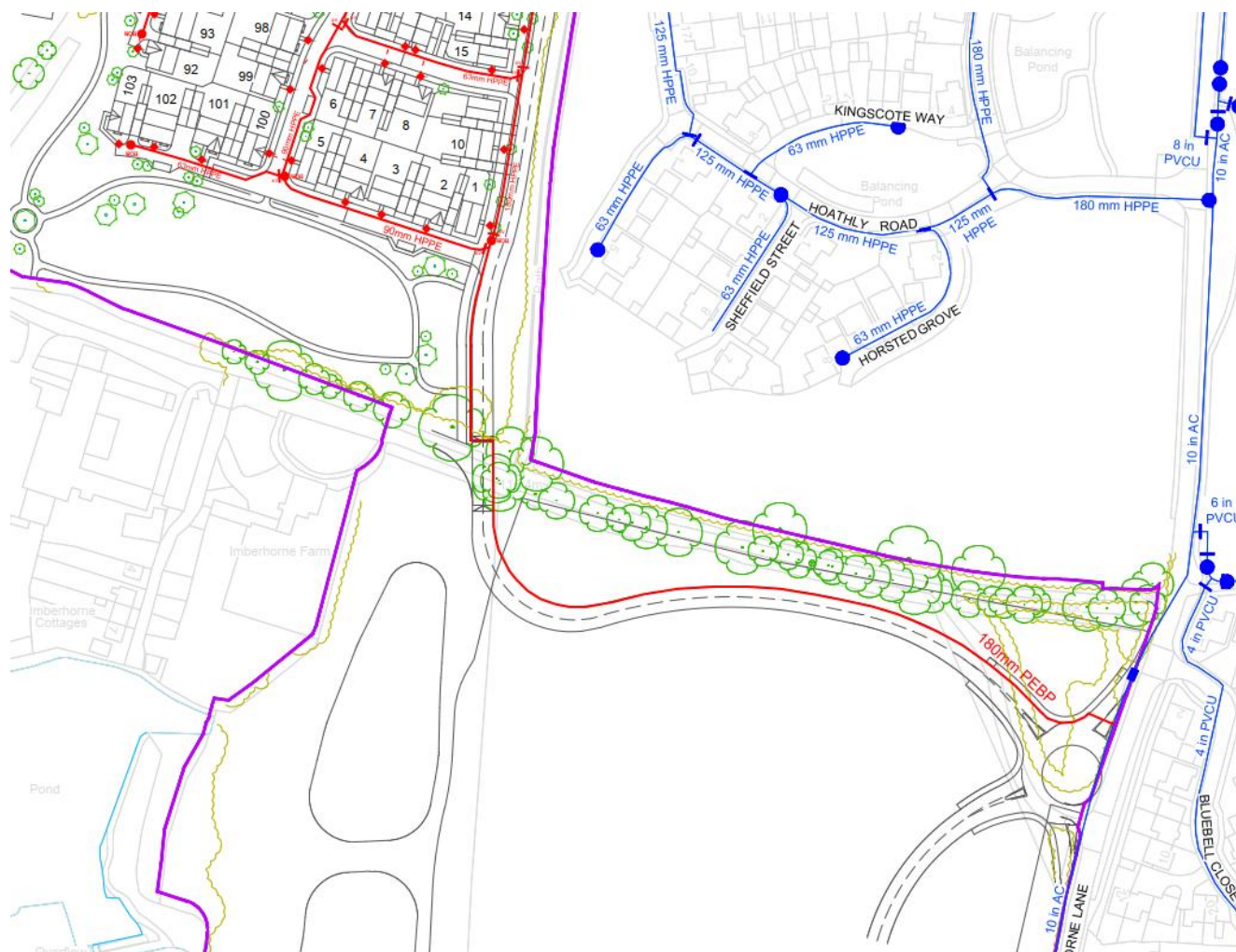
Figure 6 – Proposed Water Main Connection
