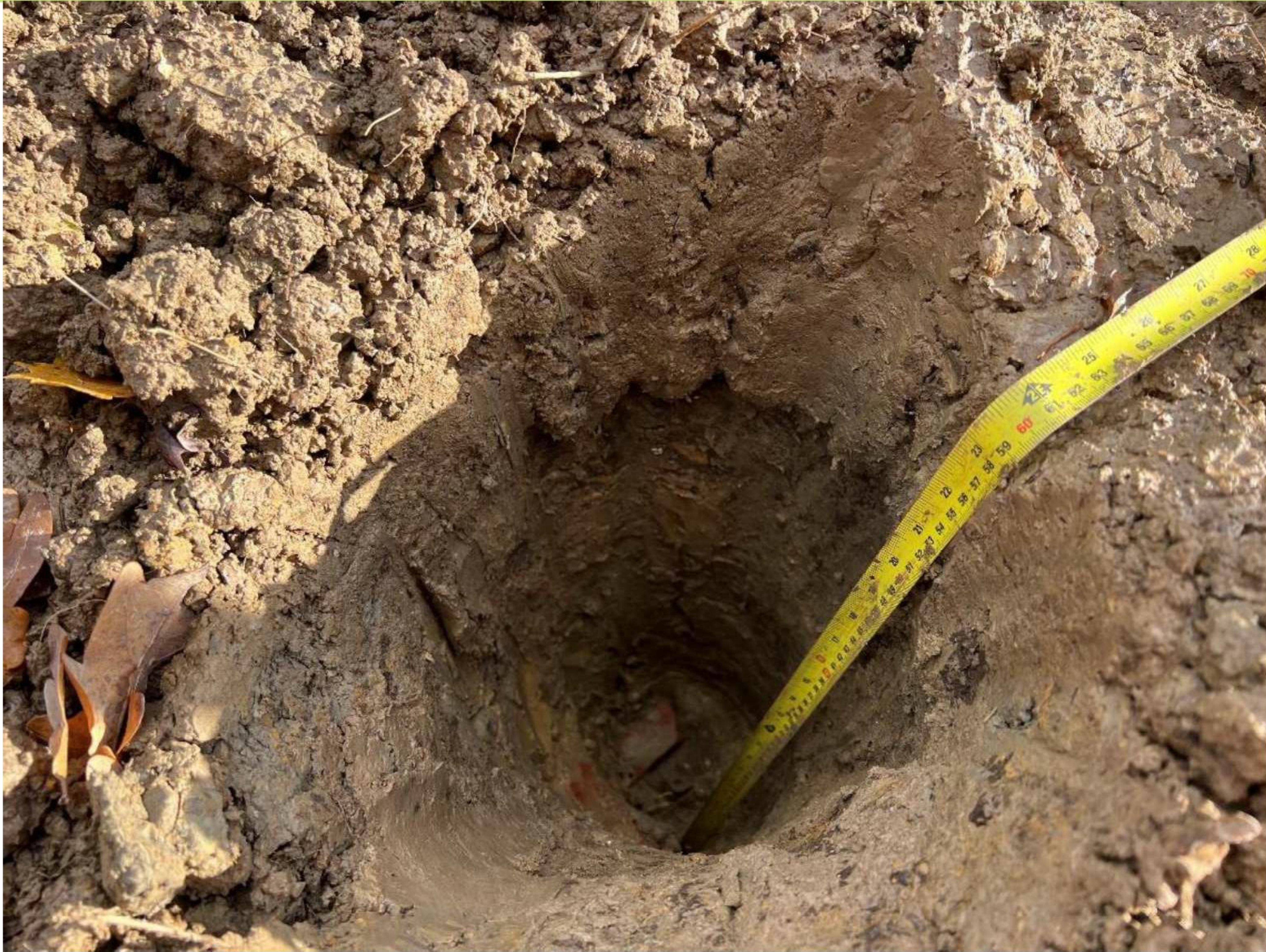
Plate 21 – Plot 3 public open space clean cover thickness recorded as 600mm (Dated 03.12.2025)
