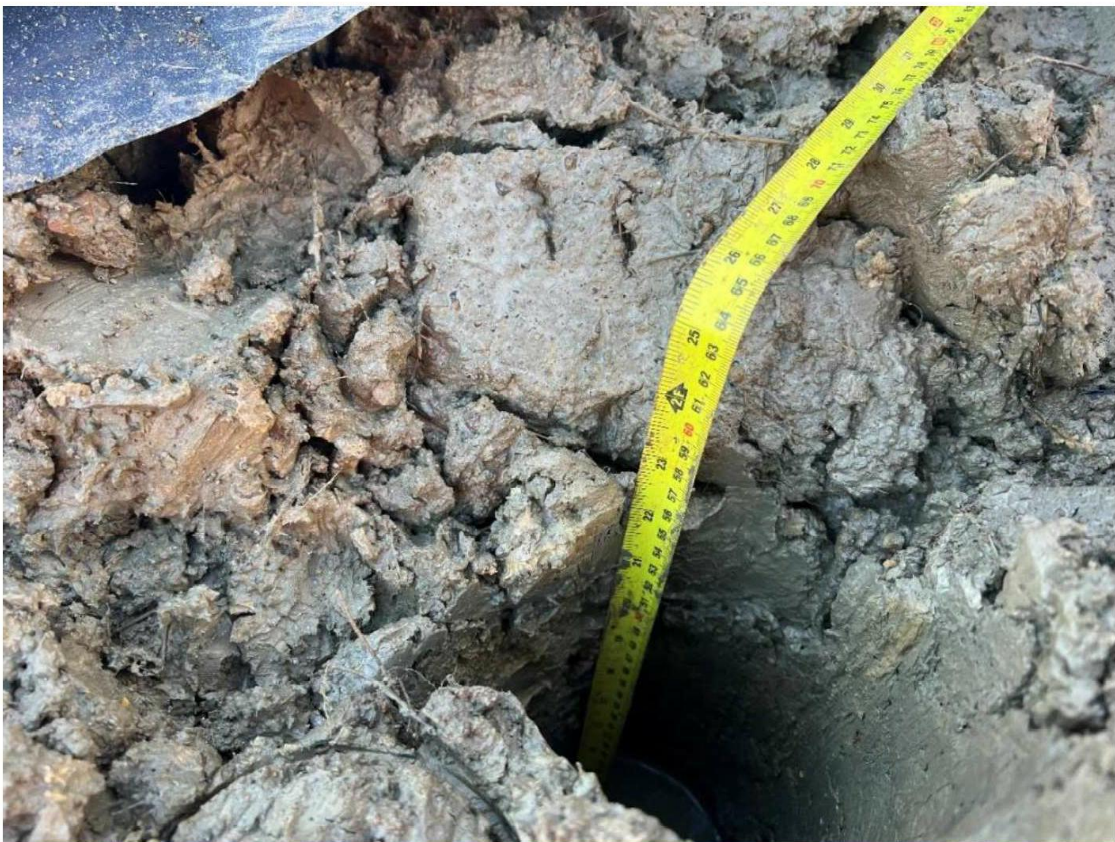
Plate 17 – Plot 4 rear garden clean cover thickness recorded as 650mm (Dated 03.12.2025)
