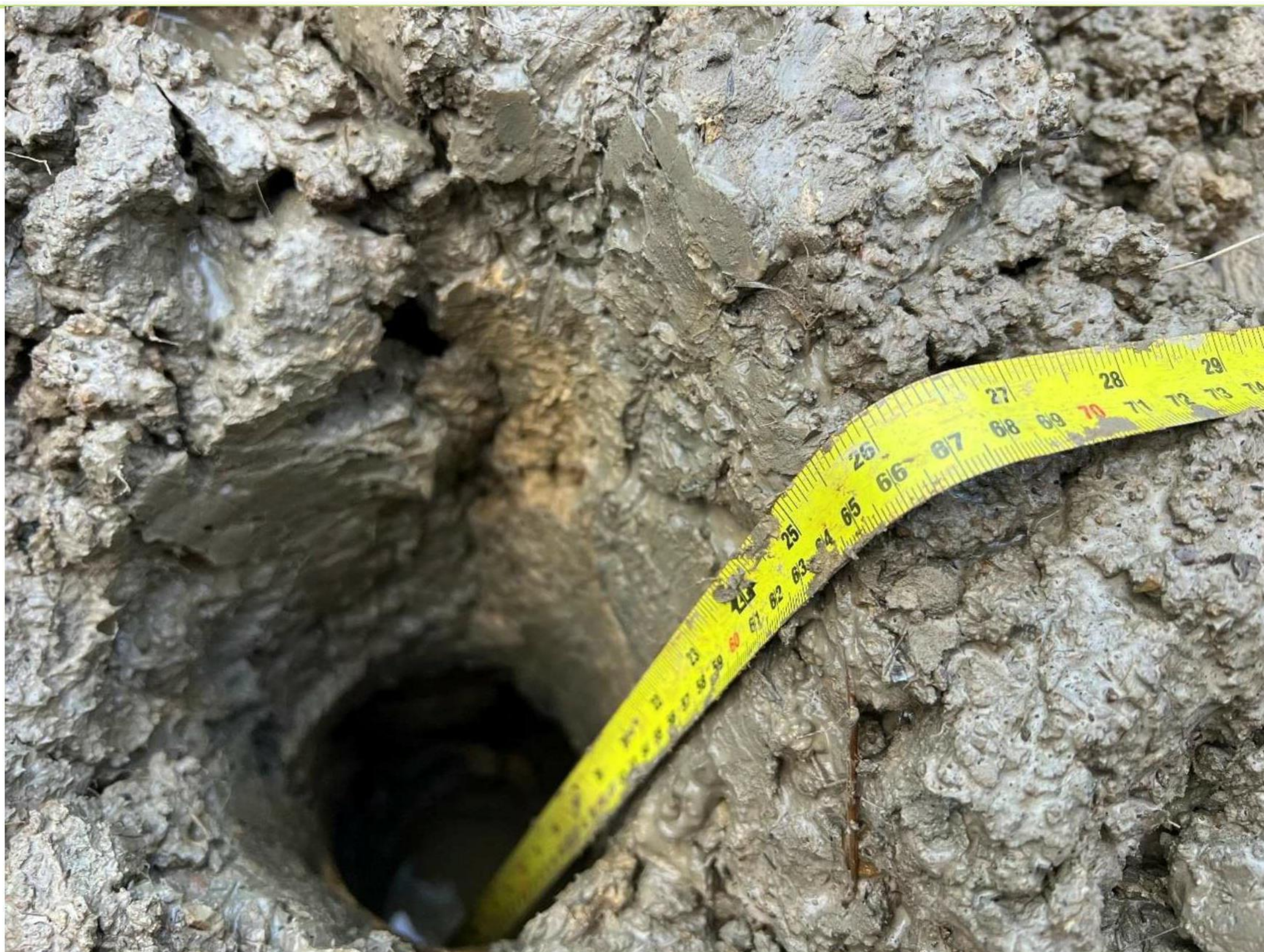
Plate 24 – Plot 34 rear garden clean cover thickness recorded as 660mm (Dated 03.12.2025)
