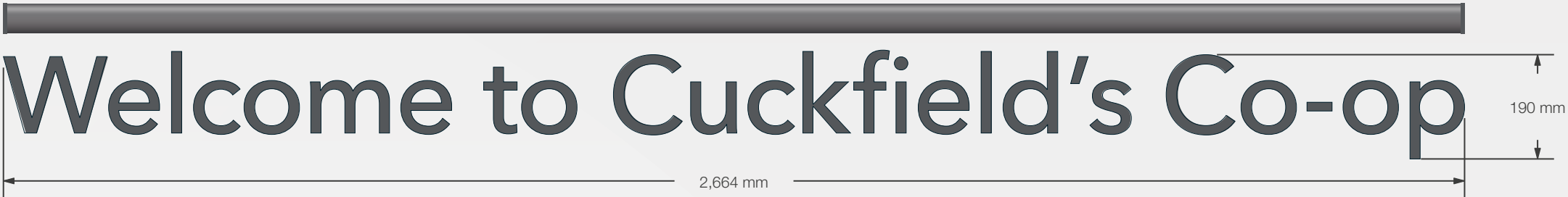
Item 2 1 No set of 5mm grey painted timber welcome letters on locators. Illuminated by new trough light Size: 2664mm span, 190mm o/a height Scale: 1:10
