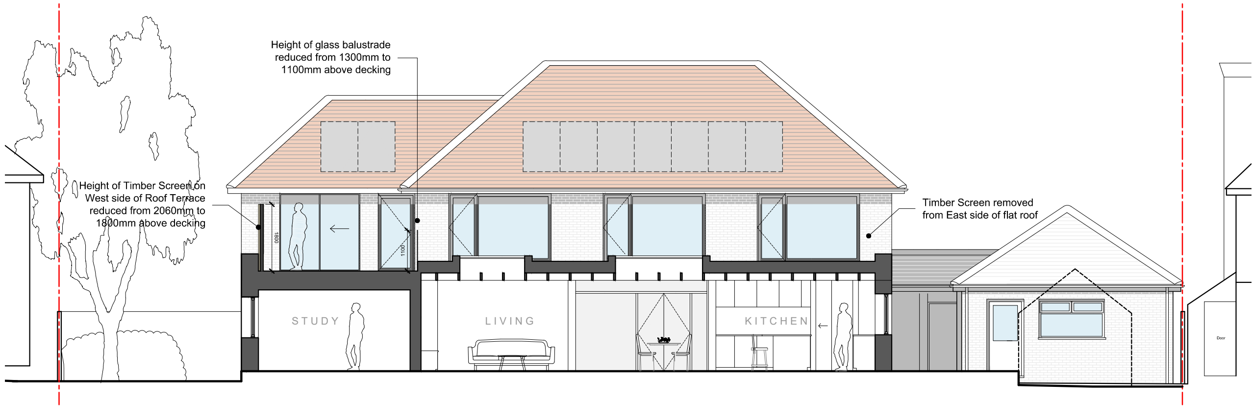
1 Section A Through GF Extension (Long) 1:100
