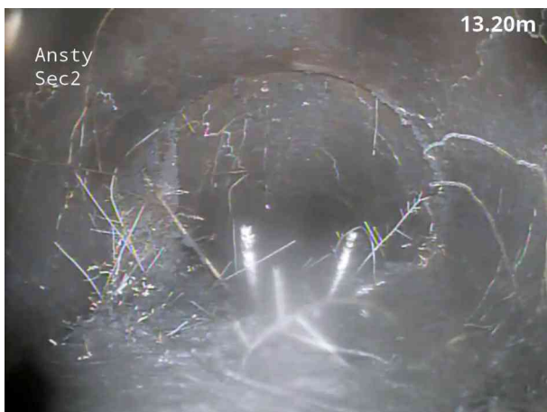
17, 00:02:07, 13.30 m Roots, mass, 30% cross-sectional area loss, change
