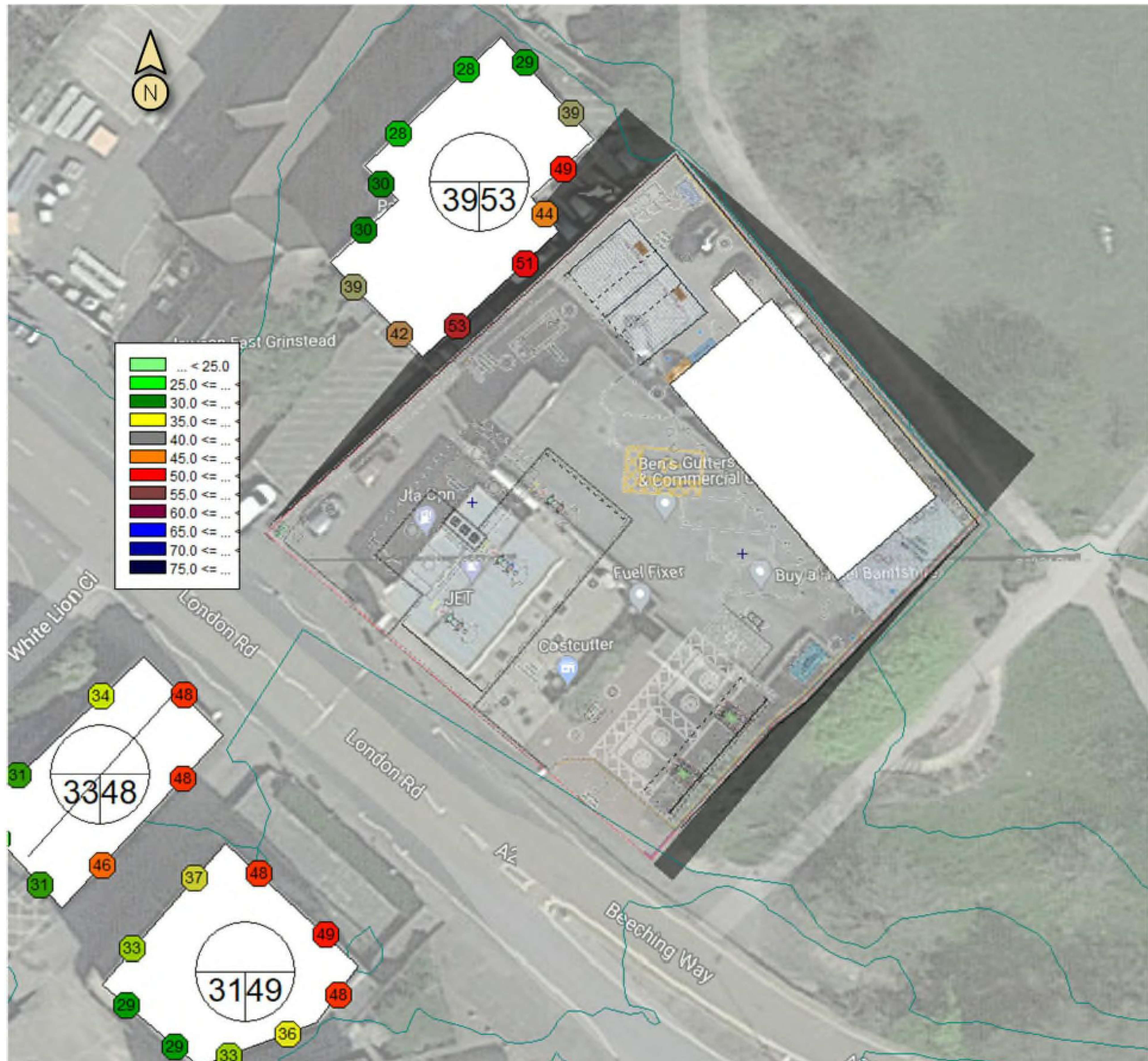
Figure 6: Calculated worst case resultant noise levels from unloading of fuel delivery and waste collection - image shows waste collection noise levels incident on facades
