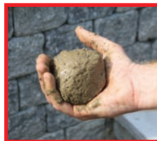
Too much moisture
