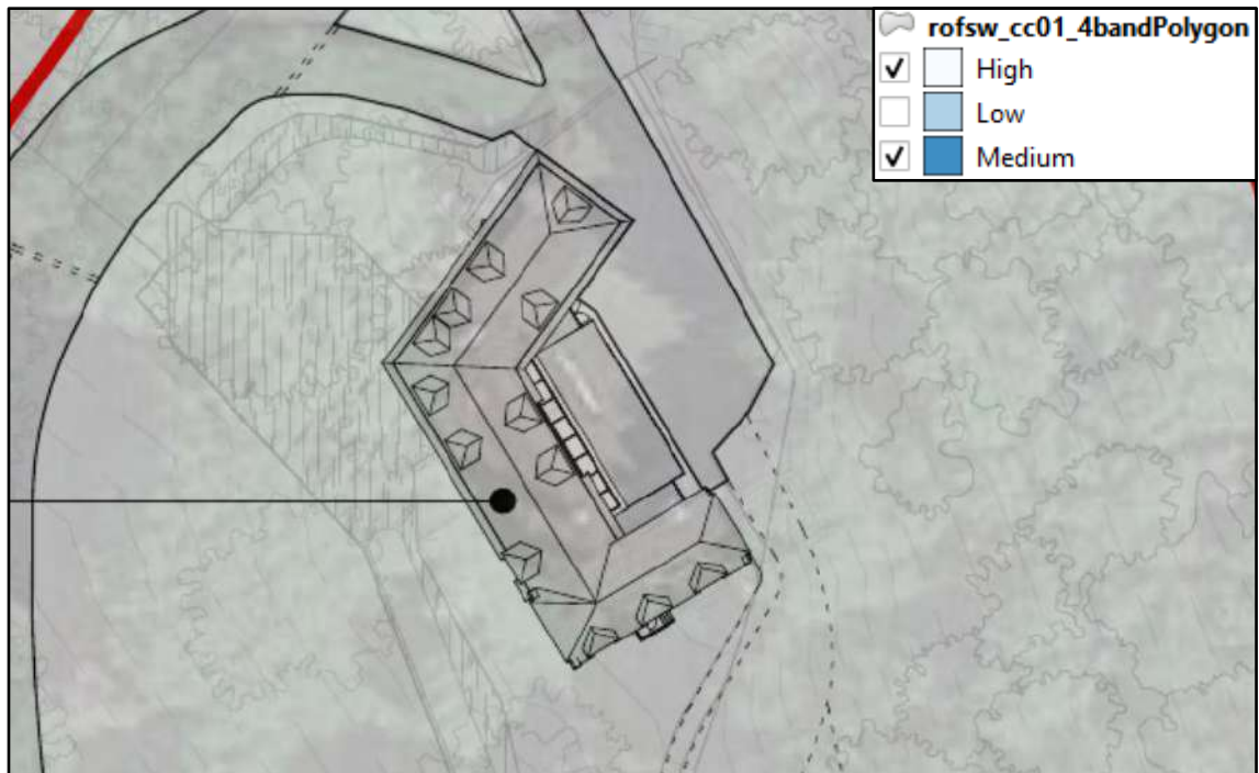
Figure 4 - Figure showing no modelled flood risk to the proposed lodge (post-works) during the 1 in 100 +CC (medium risk) and 1 in 30 +CC (high risk) storm events
