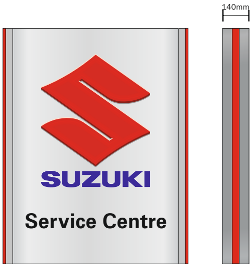
Sign D Scale: 1:20 NON ILLUMINATED Wall Mounted Sign. Fret cut aluminium panel with backed up acrylic graphics Red LED to sides NON ILLUMINATED Size - 976mm x 1275mm Cap height for 'Z' of SUZUKI = 90mm Logo height = 555mm Height from ground level: 3600mm
