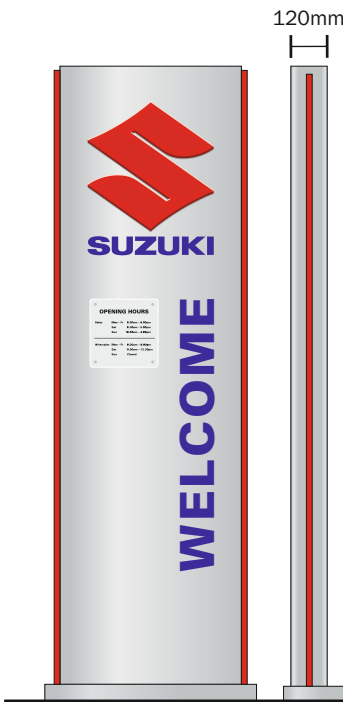
Sign 'E' Scale 1:25 Description - Single sided welcome sign Freestanding Materials - Aluminium, acrylic and vinyl Illumination - Illuminated Via LEDs Red aluminium tube edging APPROX Size - 700mm x 3000mm Cap height for 'Z' of SUZUKI = 61mm Cap height for 'W' of WELCOME = 113mm Logo height = 413mm
