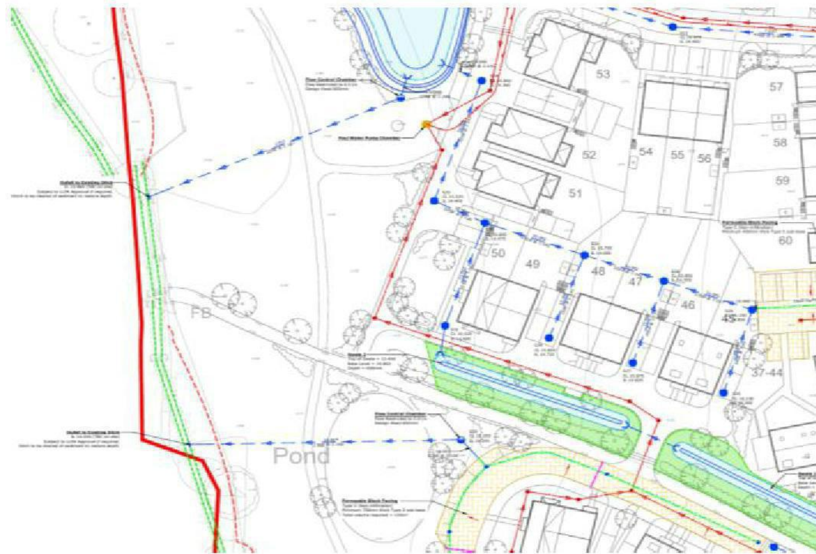
FRAADS Appendix O Site Drainage Strategy showing water being piped to 2 discharge point the stream either side of the footbridge.
