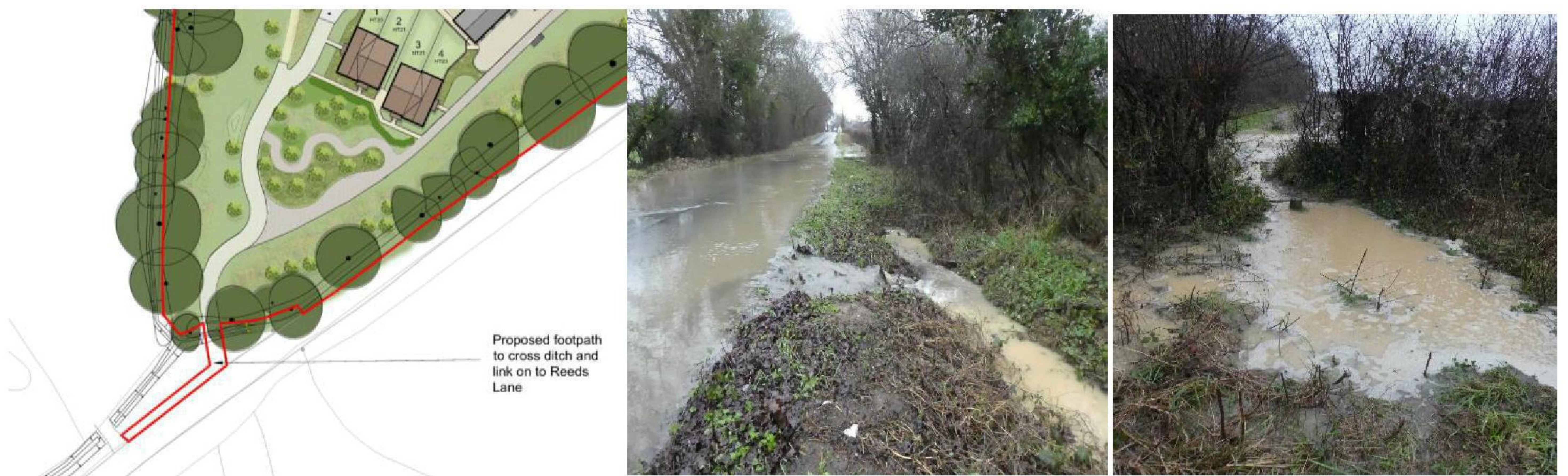
Left extract from Site Masterplan showing the new proposed footpaths at the SW site corner. Photos 05/01/2025, centre, Reeds Lane flooded at the point that the new footpath will exit onto it. Right, the flooded entrance to the southern PROW 3A1 at this point, with flood water pouring down through it onto Reeds Lane.
