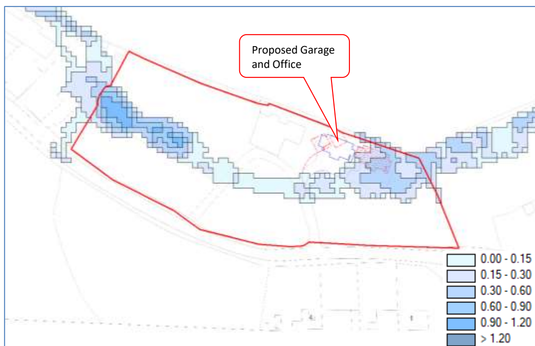
Figure 5 EA Long Term Flood Risk Maps (Depths) – High Risk of surface water flooding (source: EA Long Term Flood Risk Maps), site bordered red.
