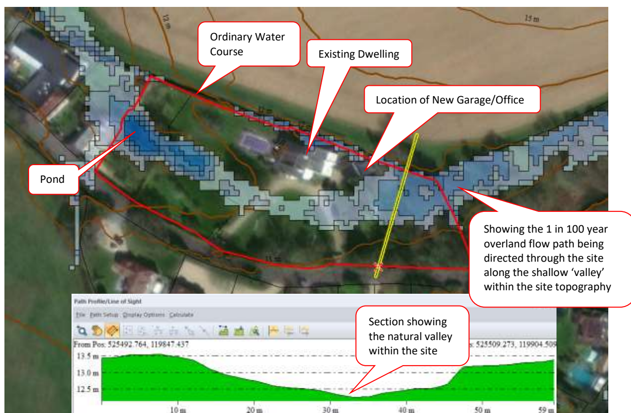
Figure 4 – Contour Map, site bordered red, yellow line represent section line of path profile (source: DEFRA Lidar Data 1m)
