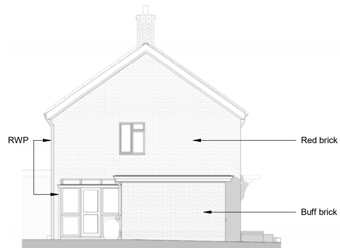
Existing South Elevation
