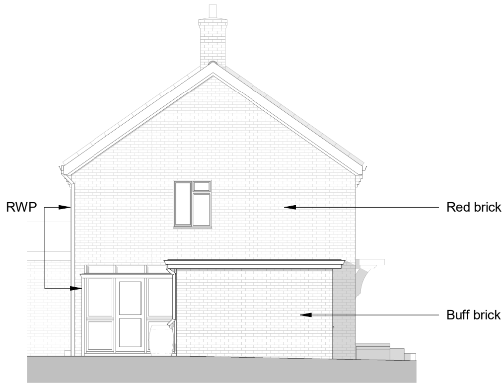
1 Existing North Elevation 1 : 100
