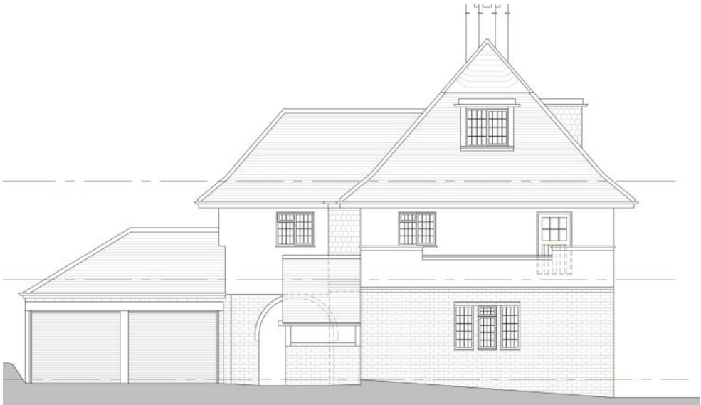
Existing West View of the House with attached double garage. Existing balcony at 1st floor (RHS)
