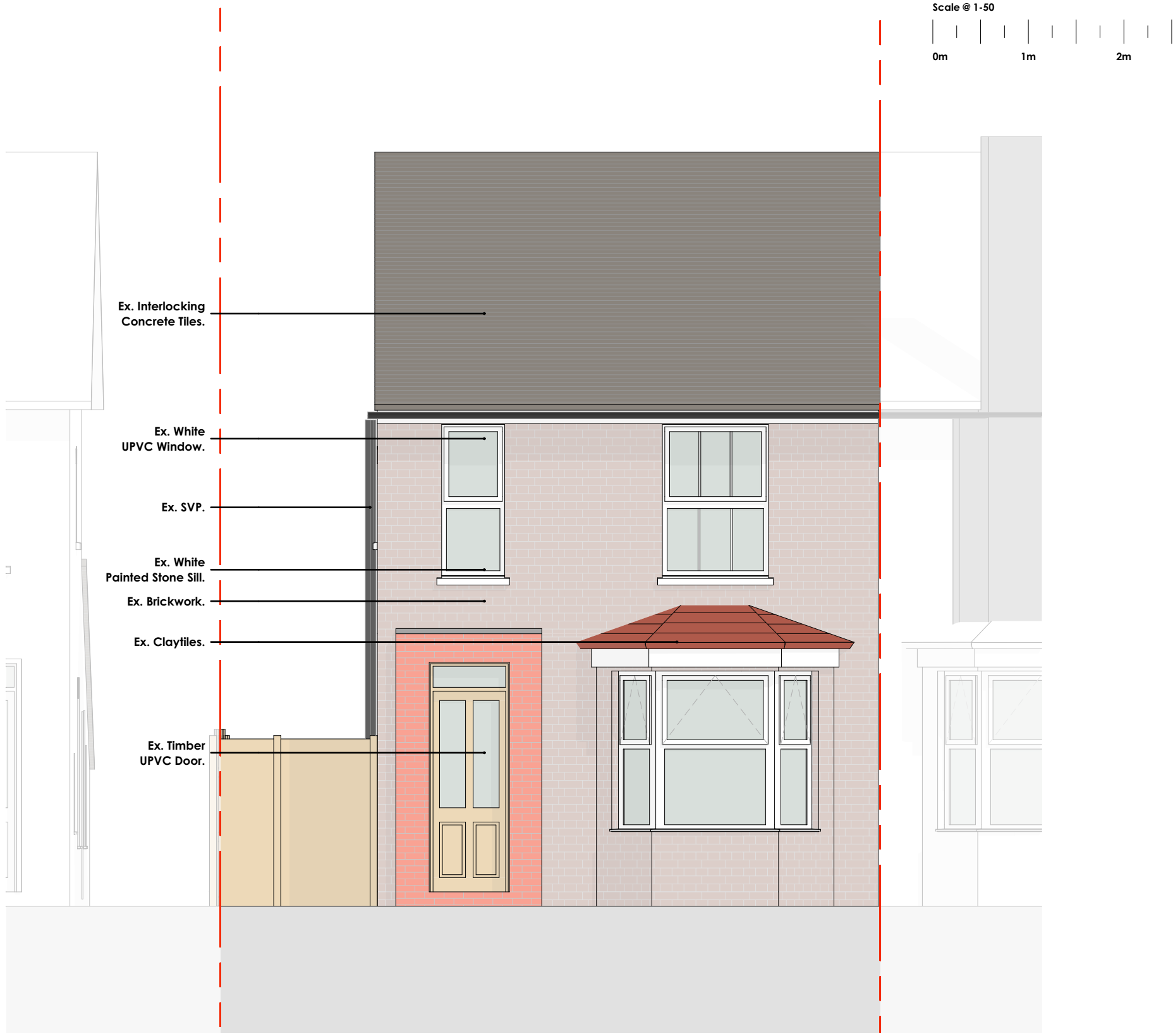
Existing East Elevation
