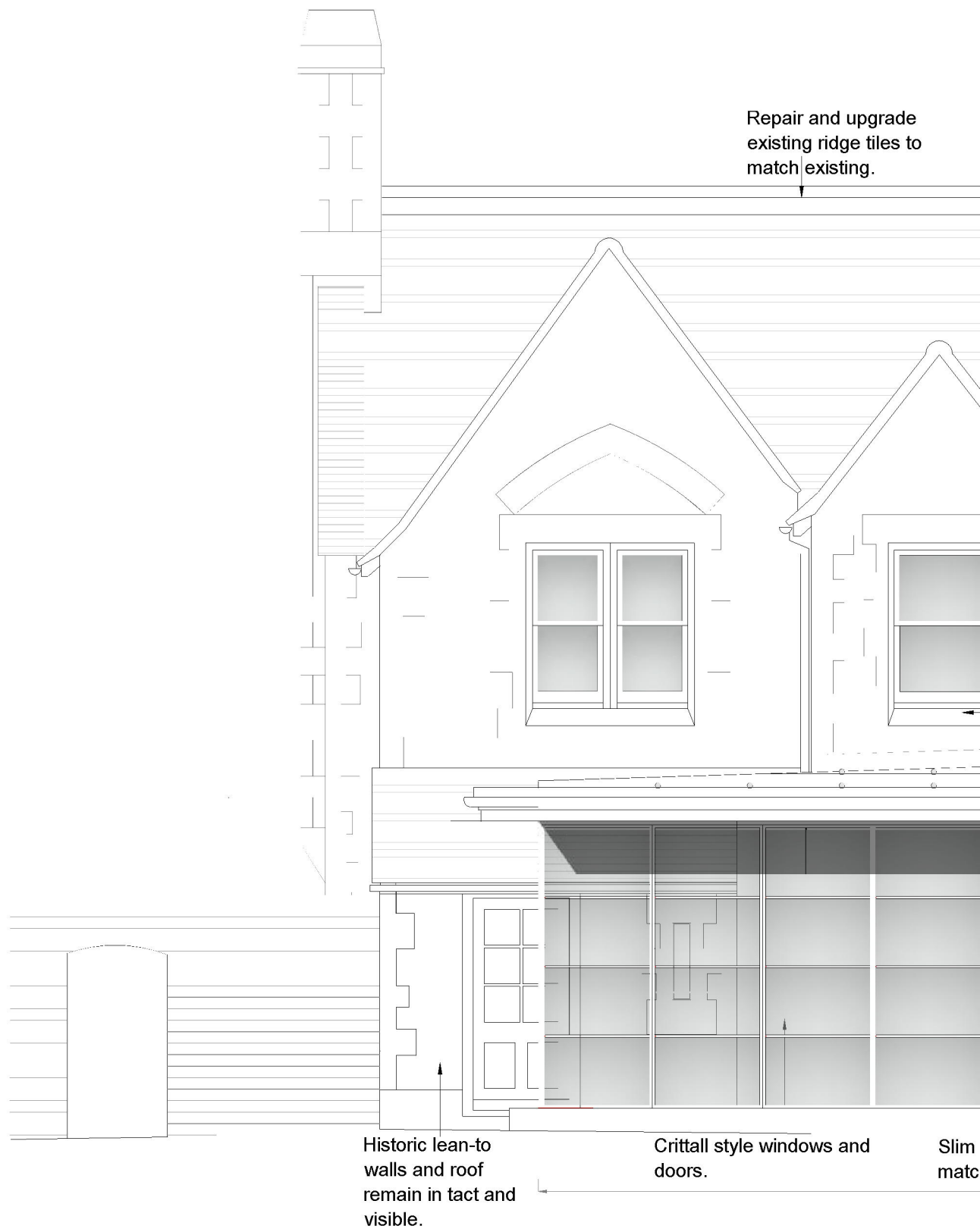
REAR ELEVATION - AS PROPOSED SCALE @ 1:50 ON AN A1 SHEET
