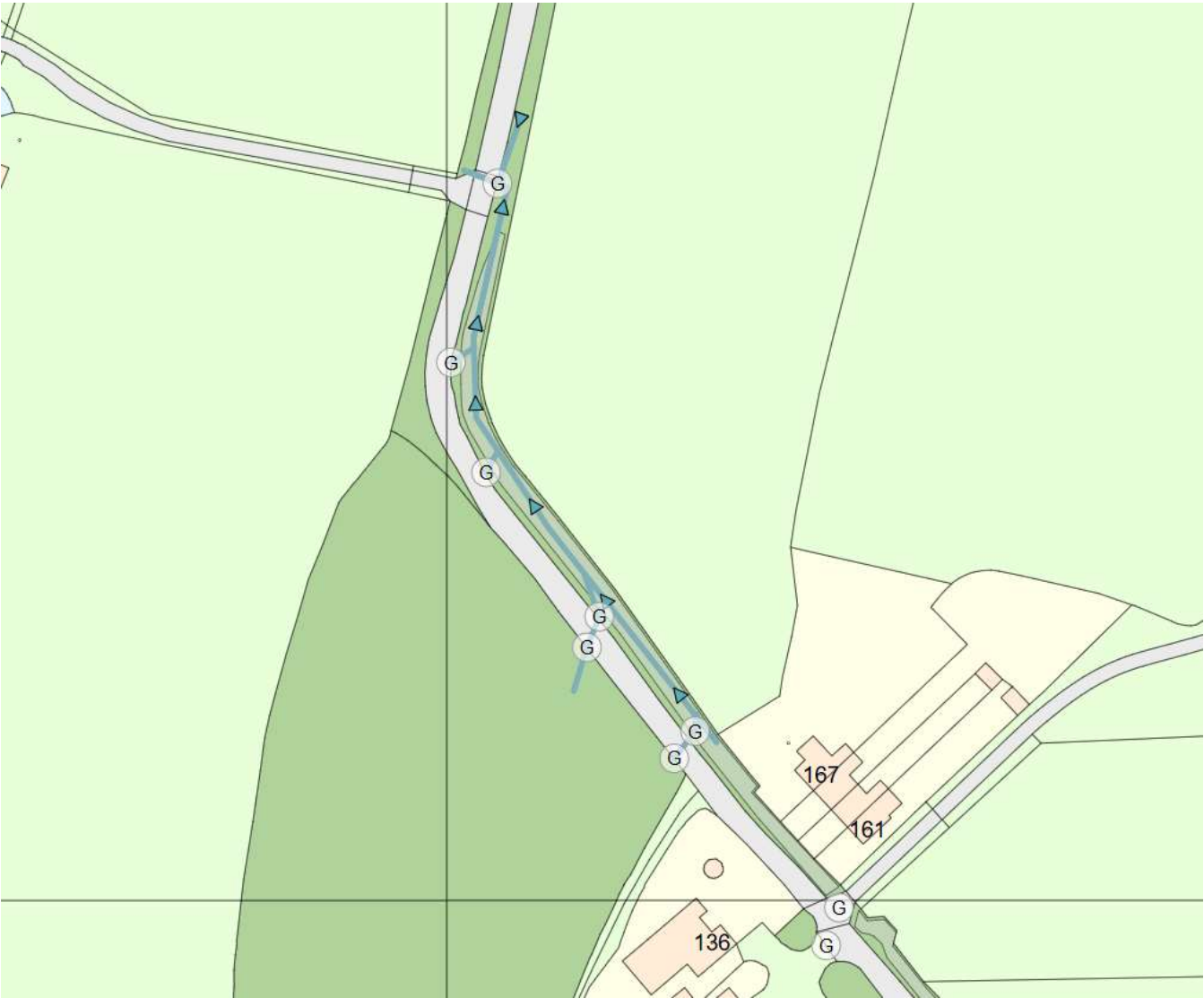
College Lane, Hassocks – Existing Drainage Layout.
