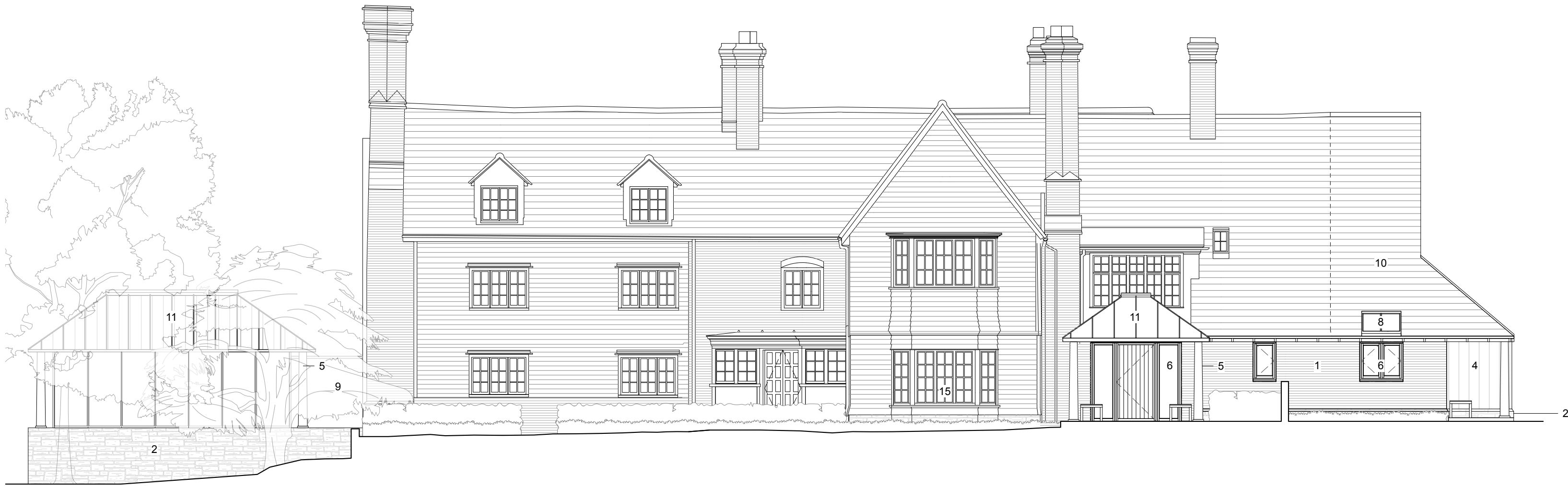
1 House-North Elevation-Proposed Scale: 1:100
