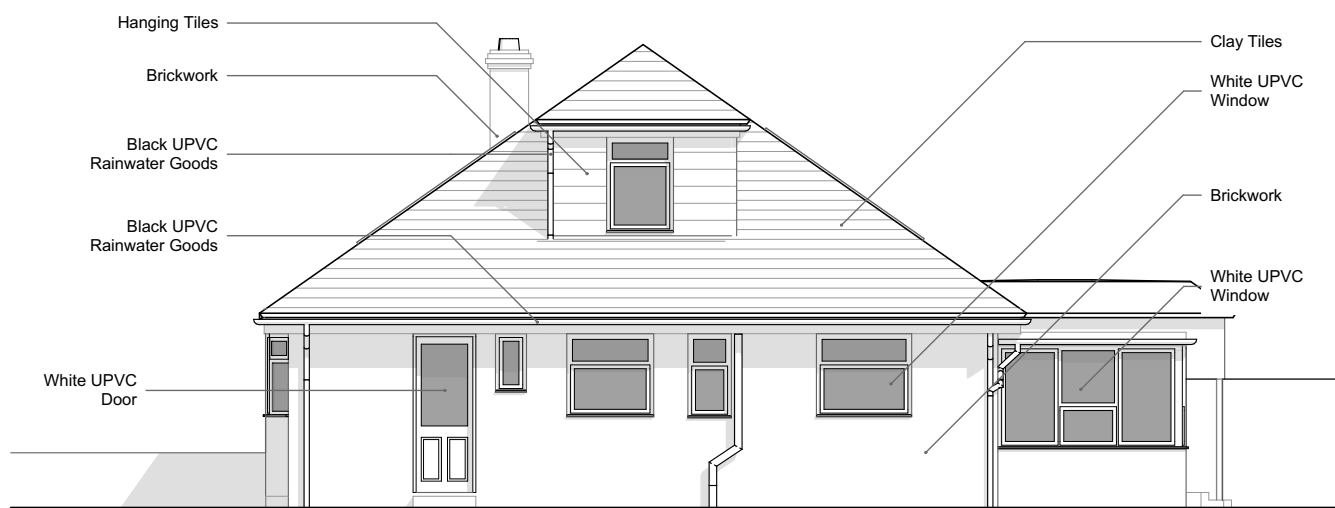
Existing North Elevation
