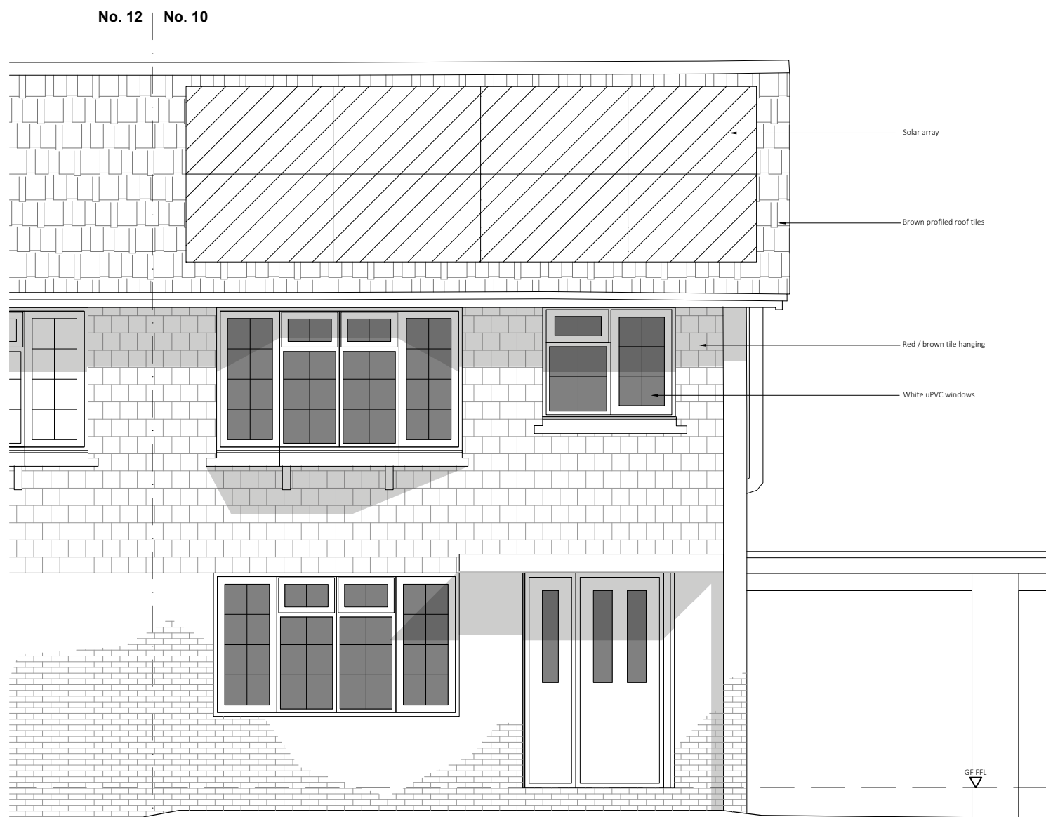
Front (South West) Elevation as Existing 1:50 @ A1
