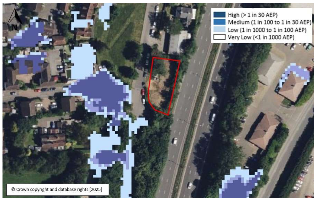
Figure 4 - Risk of Flooding from Surface Water 2050 Epoch
