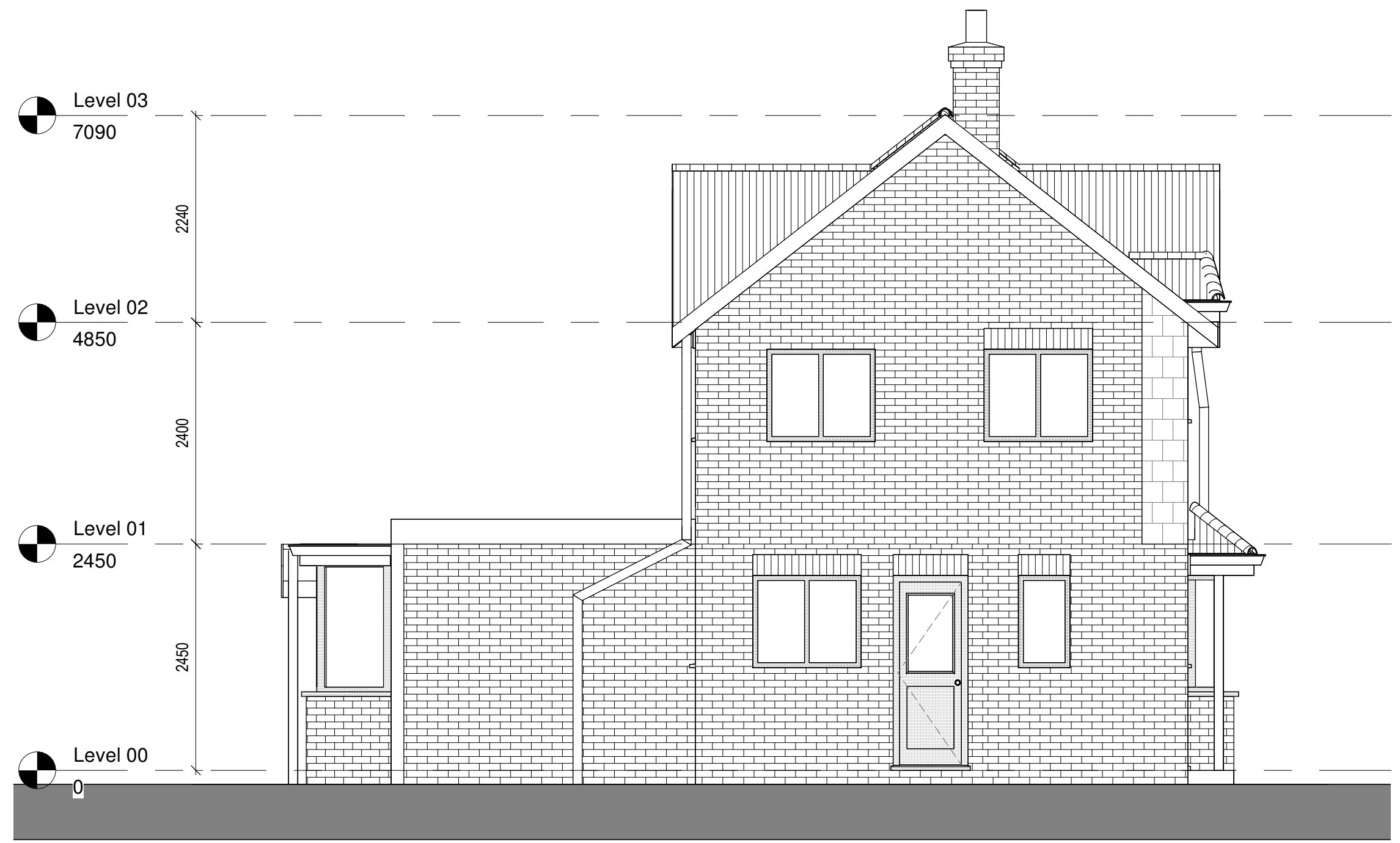
2 South Elevation - Existing 1 : 50
