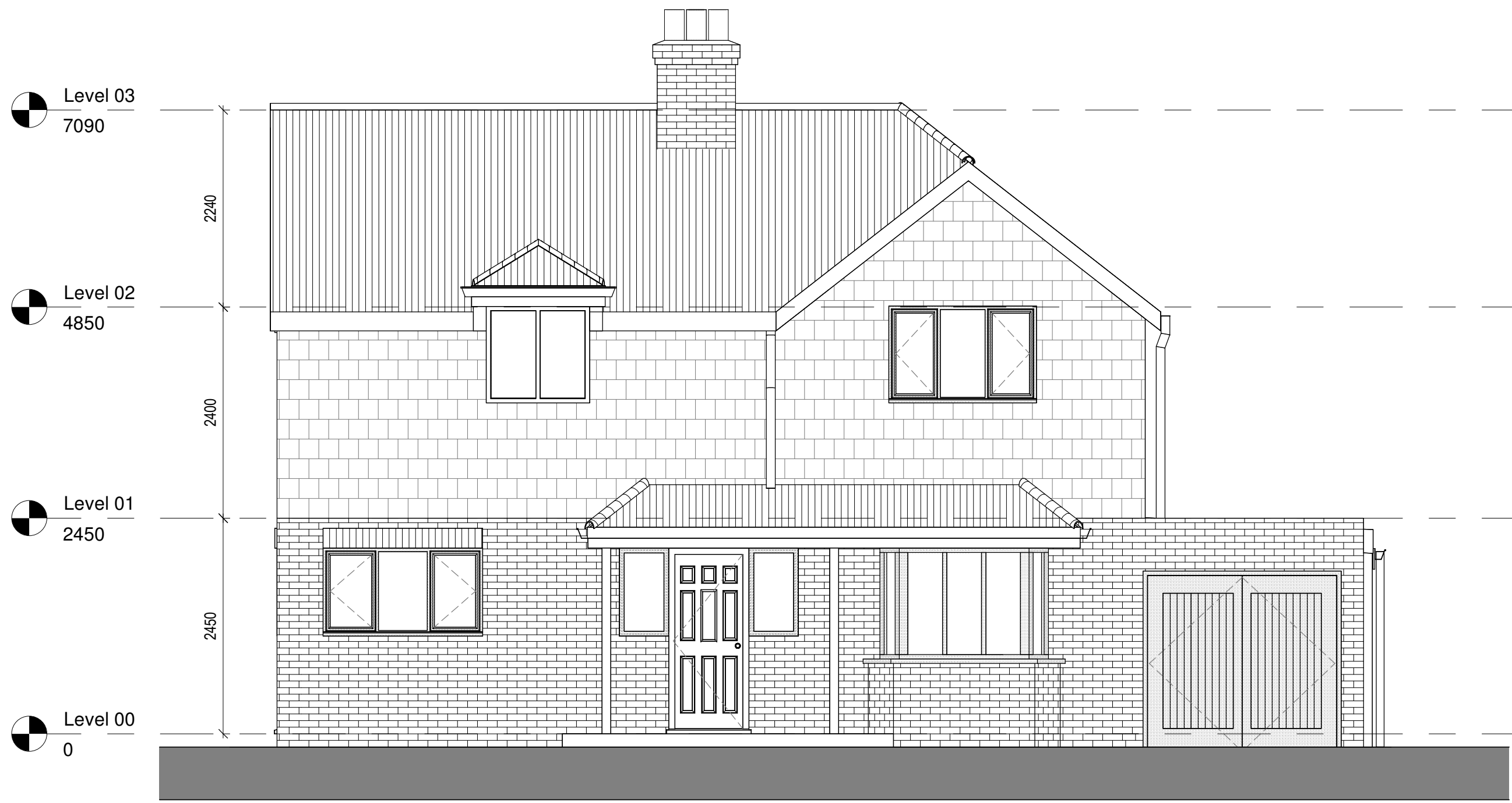
1 Front Elevation - Existing 1 : 50
